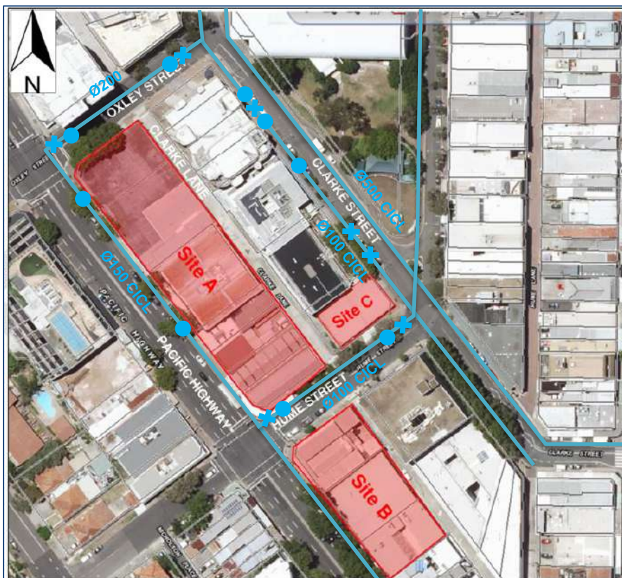
Figure 12: Existing potable water lines (solid blue lines) and sizes; existing hydrants (blue dots); existing valve (blue cross) shown (SWC, 2017)
