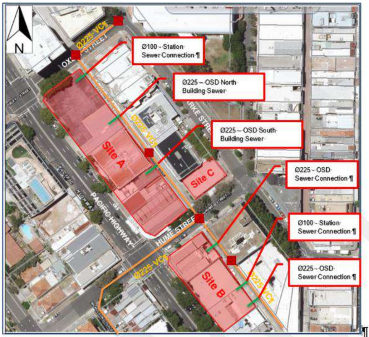
Figure 11: Existing sewerage line (solid orange lines) and size; sewerage manholes (red box); proposed station and OSD connections (solid green) indicatively shown (SWC, 2017)
