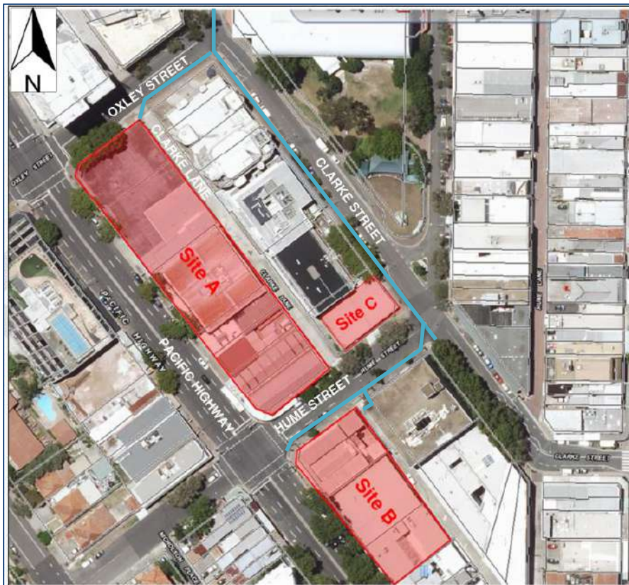
Figure 8: Existing Council Stormwater Drainage assets (solid blue lines) indicatively shown (North Sydney Council, 2017)
