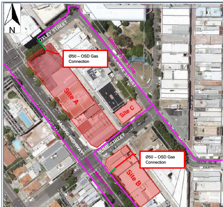
Figure 15: Existing Jemena assets (solid pink lines); proposed station and OSD connections (solid green) indicatively shown (Jemena, 2017)
