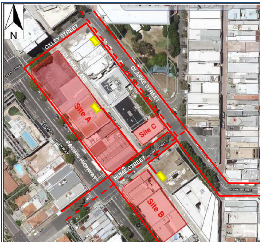
Figure 17: Existing underground cable runs (solid red lines); overhead cables (dashed red lines); pad mount substation (yellow box) indicatively shown (Ausgrid, 2017)
