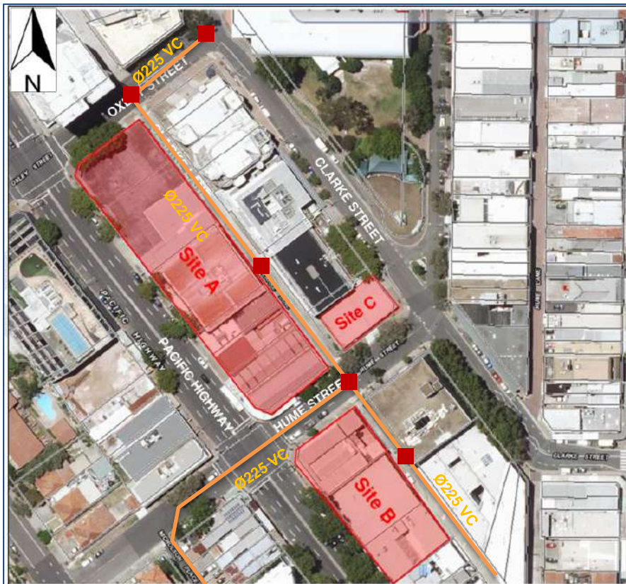
Figure 10: Existing sewerage line (solid orange lines) and size; sewerage manholes (red box) indicatively shown (SWC, 2017)
