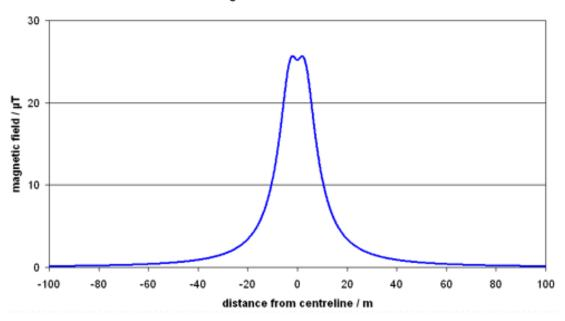
33 kV overhead line: maximum magnetic field
