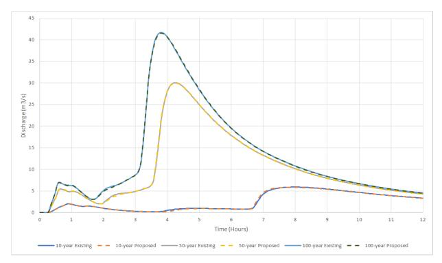
Figure 8-41: Comparison of discharge hydrographs across index section presented in Figure 8-38 (existing vs. proposed conditions)
