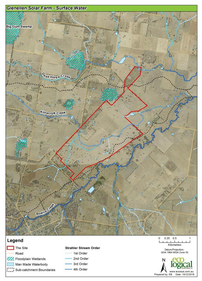
Figure 8-28: Surface water resources - drainage lines, wetlands, farm dams and Strahler Stream Order
