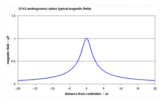
Figure 8-45: Typical magnetic field from a 33 kV underground cables (EMFs Info, 2019)
