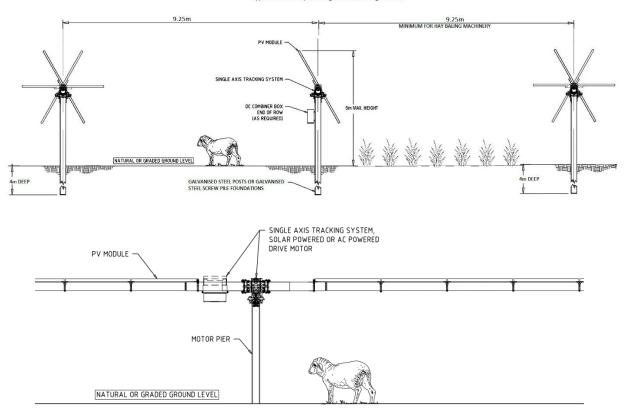
Figure 2-1: Generic Tracking System SAT elevation view showing approximate dimensions (Images courtesy of Zenviron)
