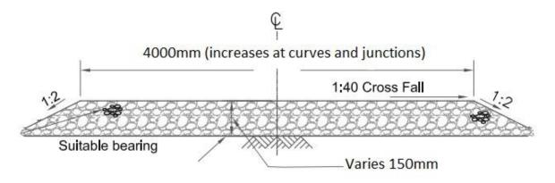
Figure 4-10: Typical track cross section
