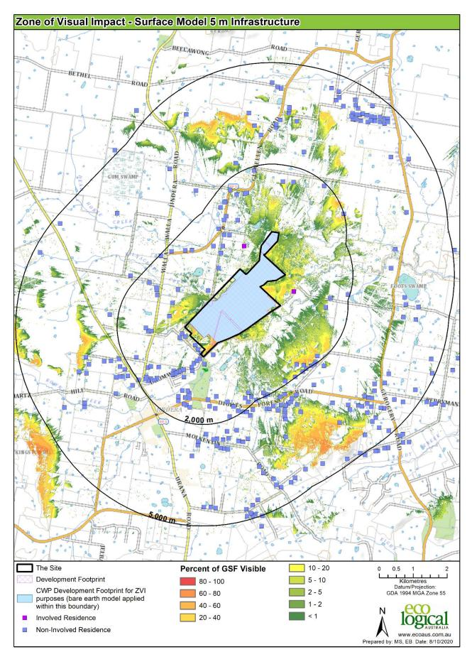
Figure 8-17: Current state surface layer ZVI for 5 m tall panel array
