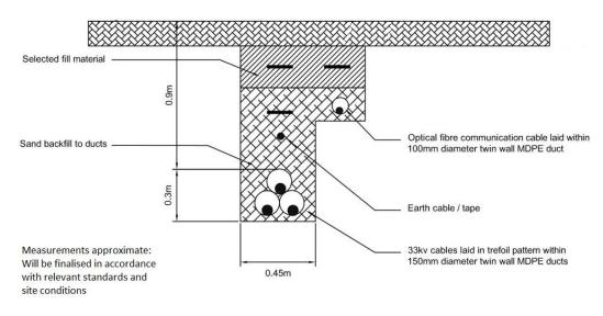
Figure 4-8: Indicative 33 kV cable trench design<sup>5</sup>
