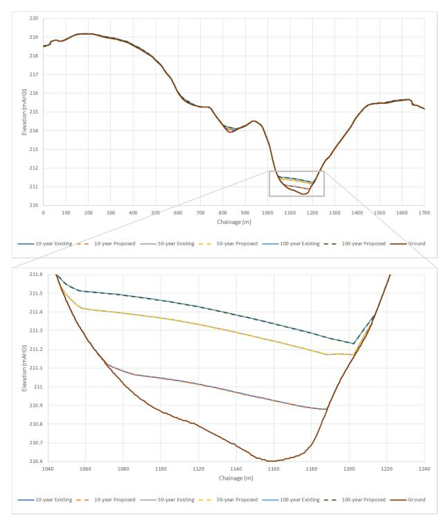
Figure 8-40: Comparison of maximum water surface elevation profiles across index section presented in Figure 8-38 (existing vs. proposed conditions)
