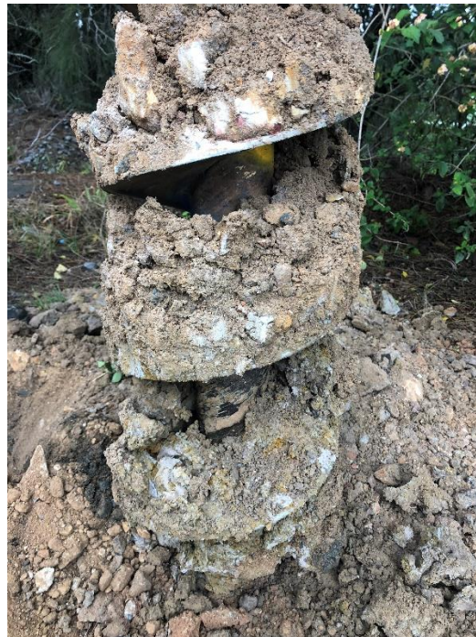
Photo 2 - Auger withdrawn from placed borehole with the sample retained
