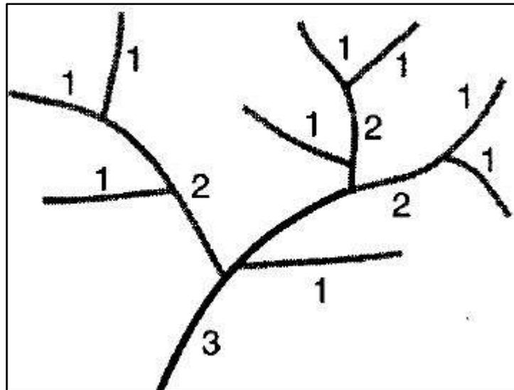
**Plate 1** Diagram showing Strahler stream order (Ritter et al. 1995, p.151)
