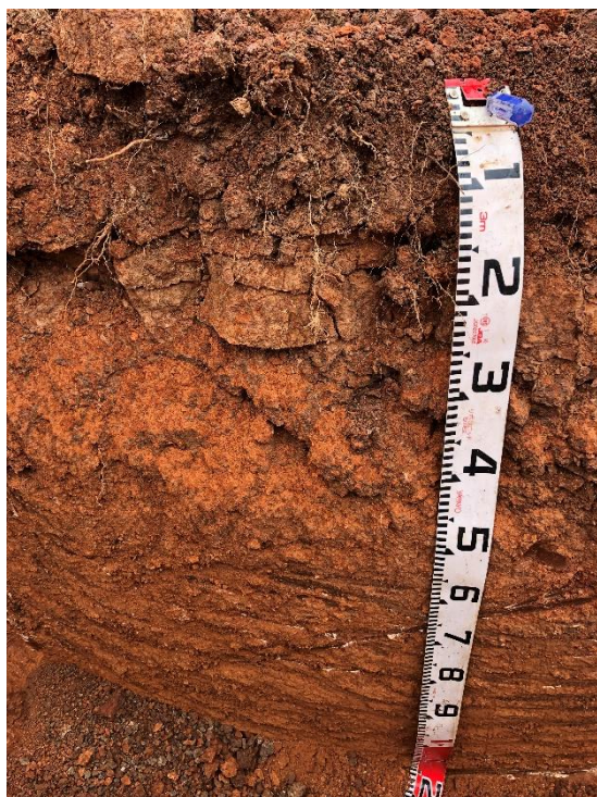
Figure 2: Typical soil profile with A and B horizons, showing carbonate in the B Horizon.
