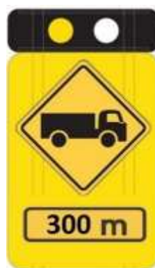
Figure 9 - Fog Activated Sign
