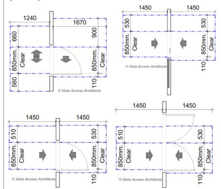
Note that the circulation spaces (other than doorway threshold ramp) to have a maximum floor grade of 1:40. Where there is a level difference at the door threshold, the maximum level difference can be 35mm if provided with a 1:8 doorway threshold ramp.
