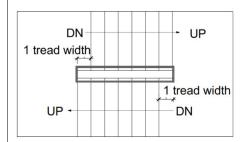
**Note:** For stairways with 90° to 180° turns at landings, in order for the handrails to comply with the consistent height requirement, the risers have to be offset at the mid-landings OR provided with a 300mm handrail extension, so that no vertical sections are created in the handrails. This applies to both non-fire-isolated and fire-isolated stairways.
