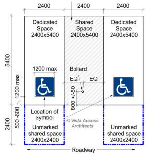
The Accessible parking, shared zones, linemarking and bollards to be as shown above.
