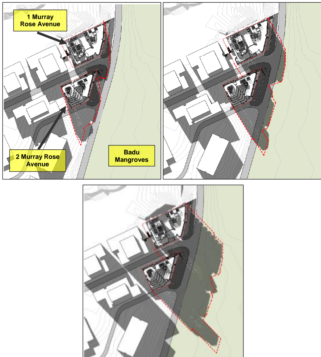
Figure 33 | Midwinter shadow diagrams (top left: 1pm; top right 2pm; bottom 3pm). Shadow from a height compliant development shown dotted red (Source: Applicant's EIS)
