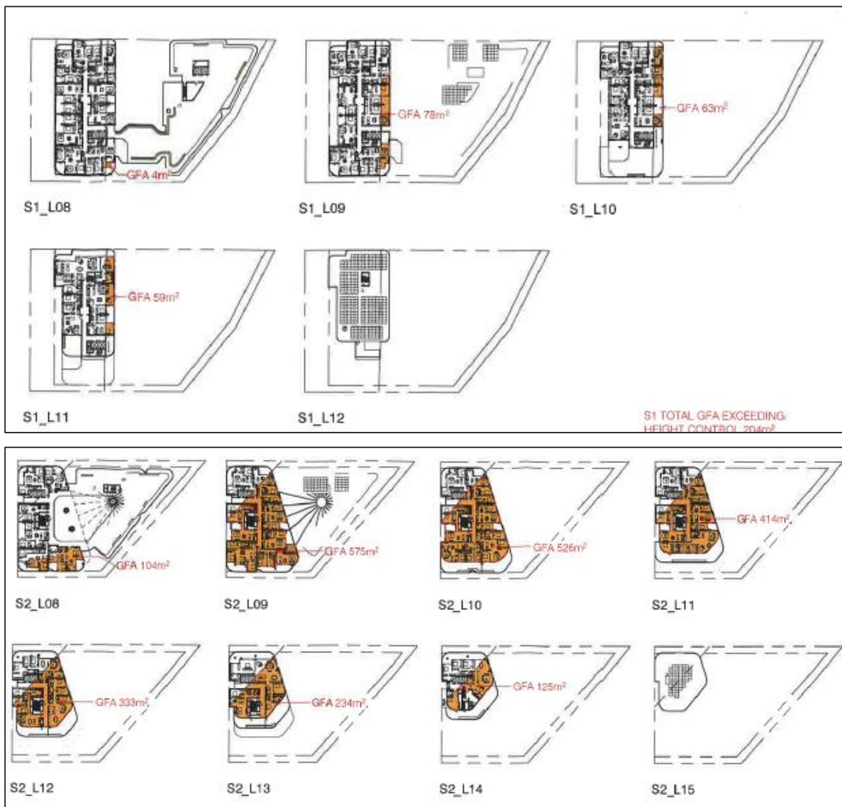
Figure 18 | Floorplans of each building with areas above the maximum height controls highlighted orange. Top: 1 Murray Rose Avenue. Bottom: 2 Murray Rose Avenue (Source: Architectural Plans)
