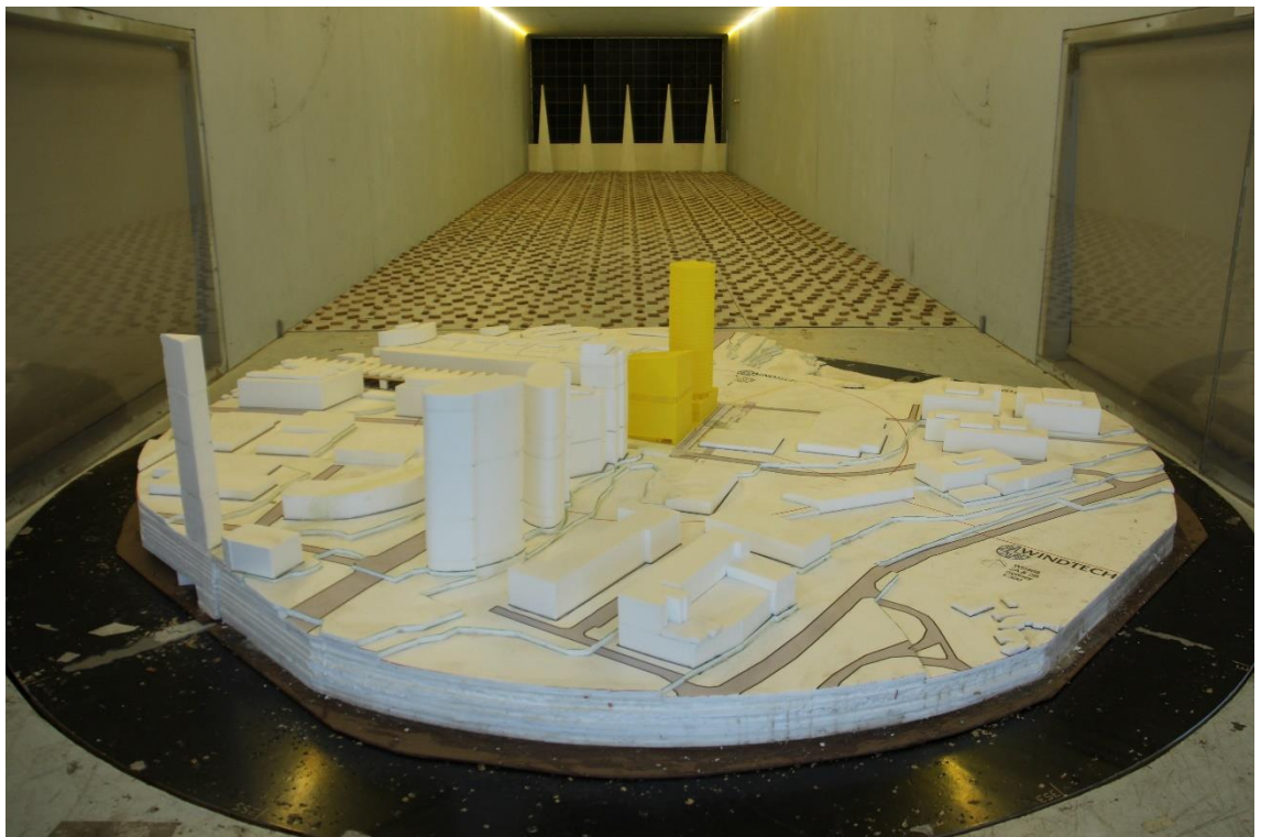
Figure 1a: Photograph of the Wind Tunnel Model – Proposed Surrounds Scenario (view from the south-east)
