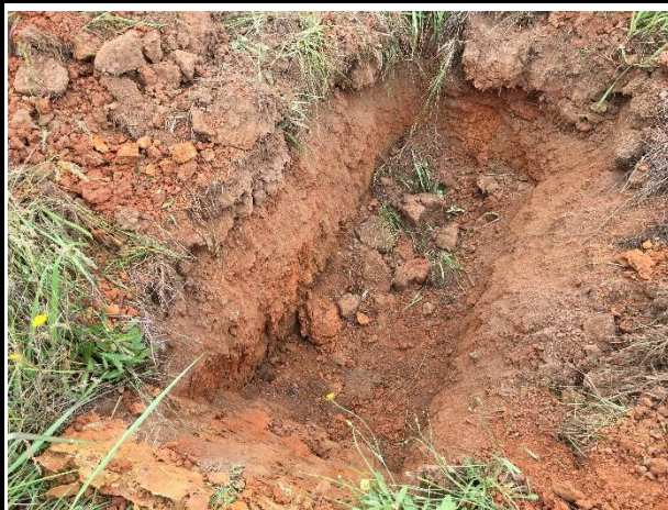
Photo 11. TP6 – minimal upper layer of silt, followed by clay characteristic of the site.
