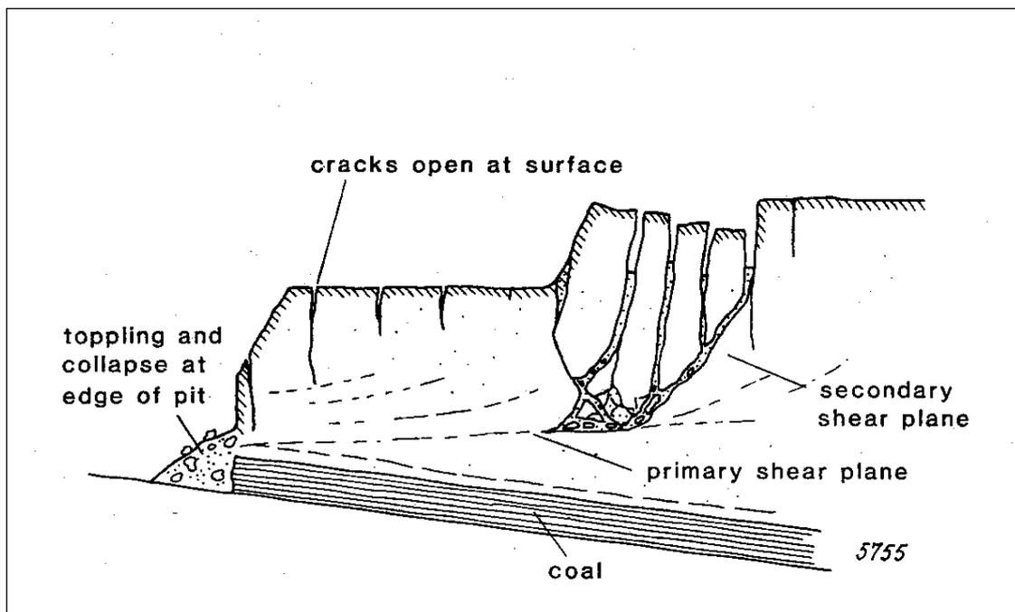
**Figure 14A – Highwall Damage Due to Adjacent Blasting (after CSIRO 1983 Report)**
