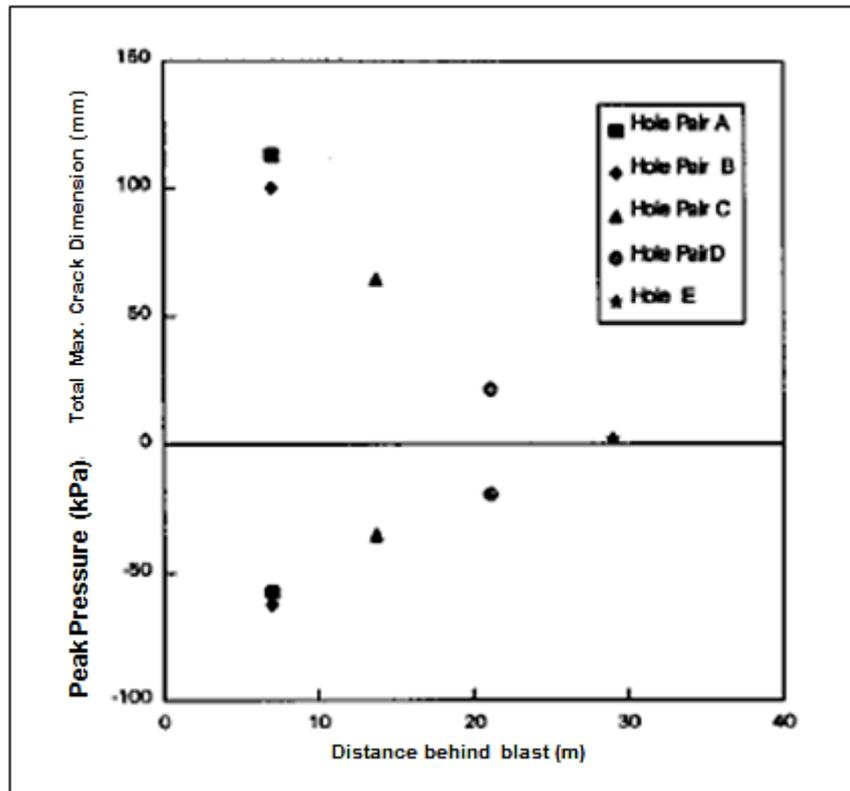
**Figure 20 – Correlation of Negative Pressures and Visible Fractures (after Brent and Smith 1996)**
