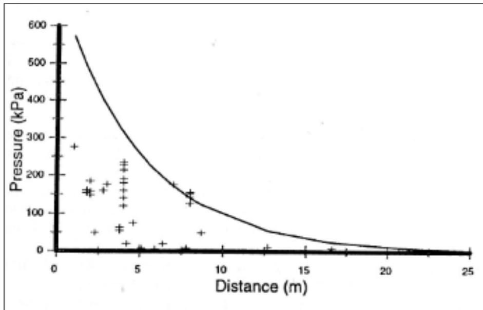
**Figure 19 – Gas Pressure Measured versus Distance – Obtained from Literature Review (after McKenzie 1999)**
