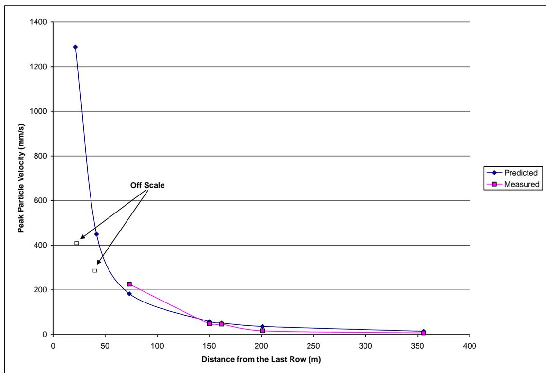
**Figure 16 – Measured versus Predicted Vibration Behaviour**
