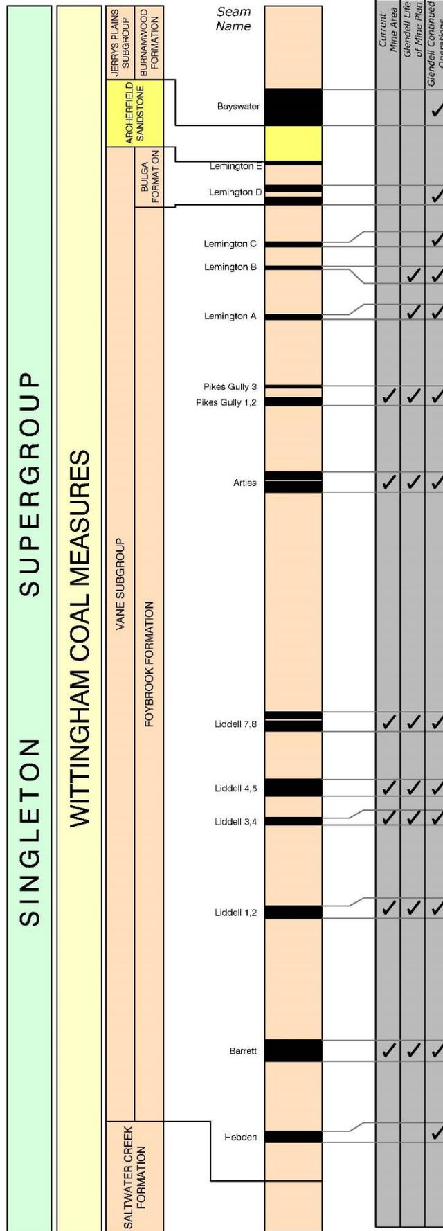
Figure 2 – Typical stratigraphy at Glendell Mine
