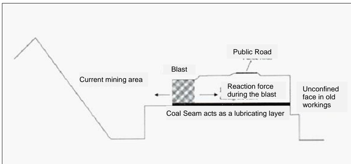
**Figure 13 – A Simplified Cross-section Showing the Risk of Bulk Displacement of the Road Bearing Pillar as a Result of Reaction Forces from the Blast on the West Side (left) of the Road (after Rorke and Thabethe, 2004)**
