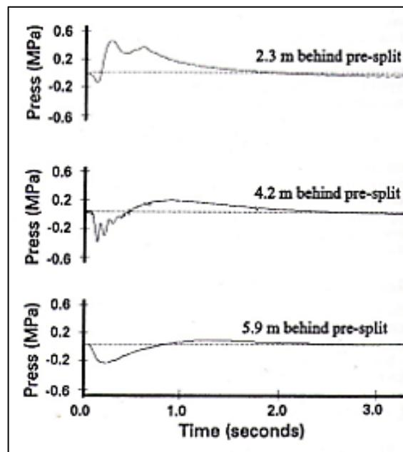
**Figure 18 – Example of Gas Pressure Waveforms Measured at Various Distances Behind Pre-split Charges (after McKenzie 1999)**
