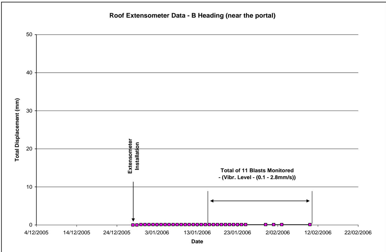
**Figure 17C – Roof Extensometer Data near the Portal Entry**
