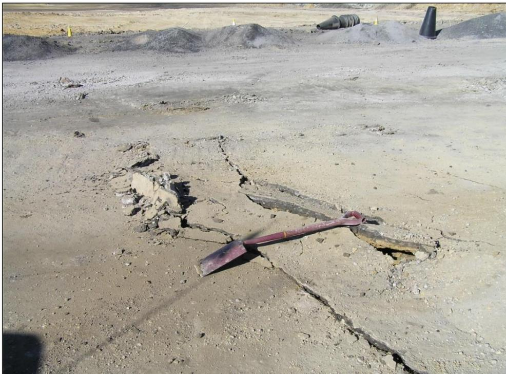
**Figure 15 – Impact of Blasting – Showing Surface Rock Strata Damage to Blasted Pre-Split Line; Extending up to 17 m from the Edge of the Blast (after Lewandowski and Cope 2009),**
