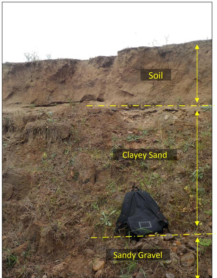
**Figure 11 – Typical Cross-section through the Creek Bank (Sept. 2018)**
