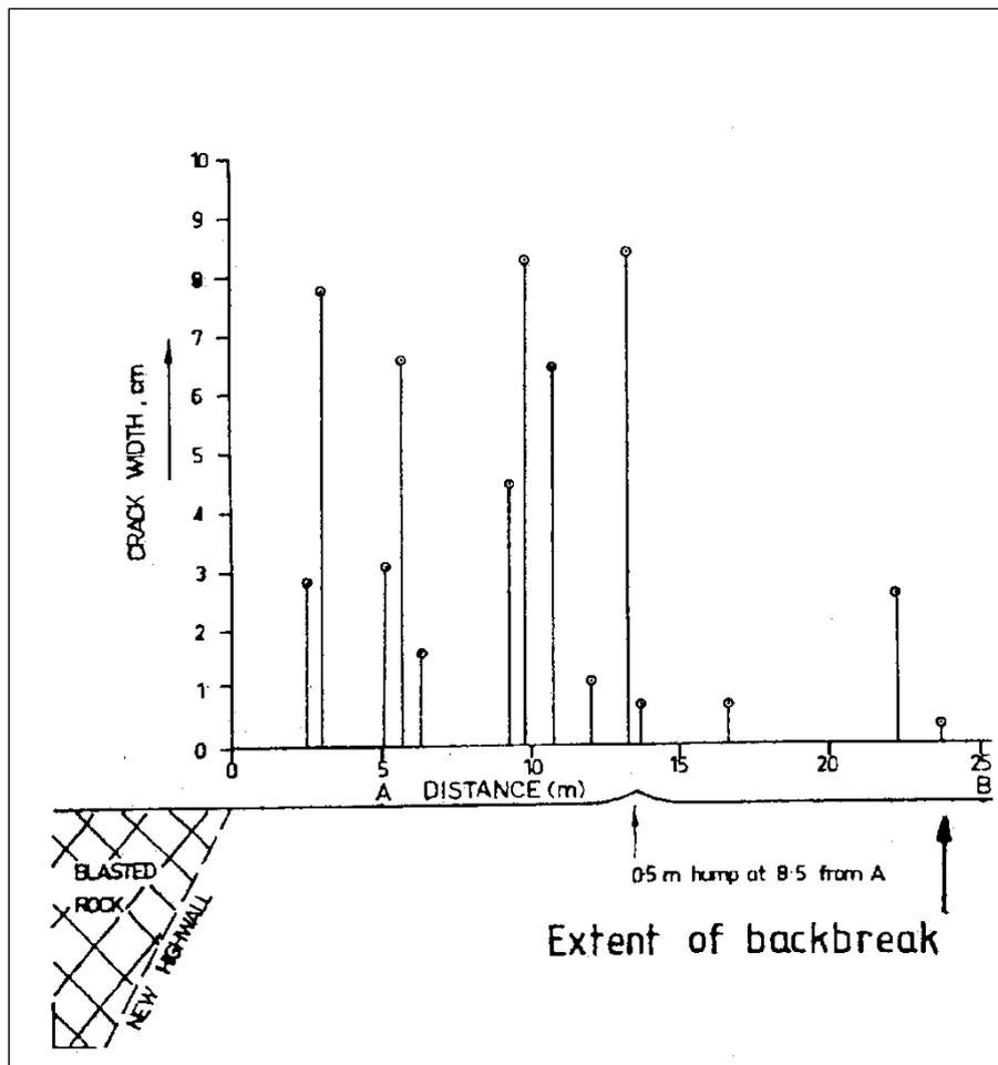
Figure 14C – Estimation of Back-break Cracking (after CSIRO 1983 report)
