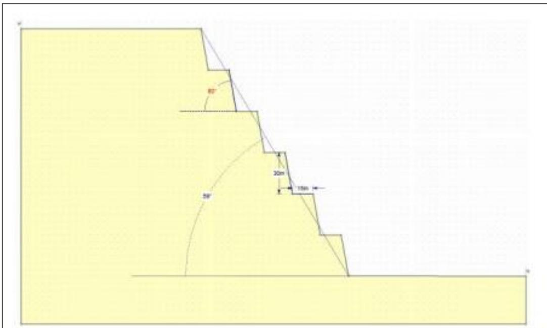
**Figure 5 – Highwall Design Criteria for Glendell Mine (after AECOM 2018)**
