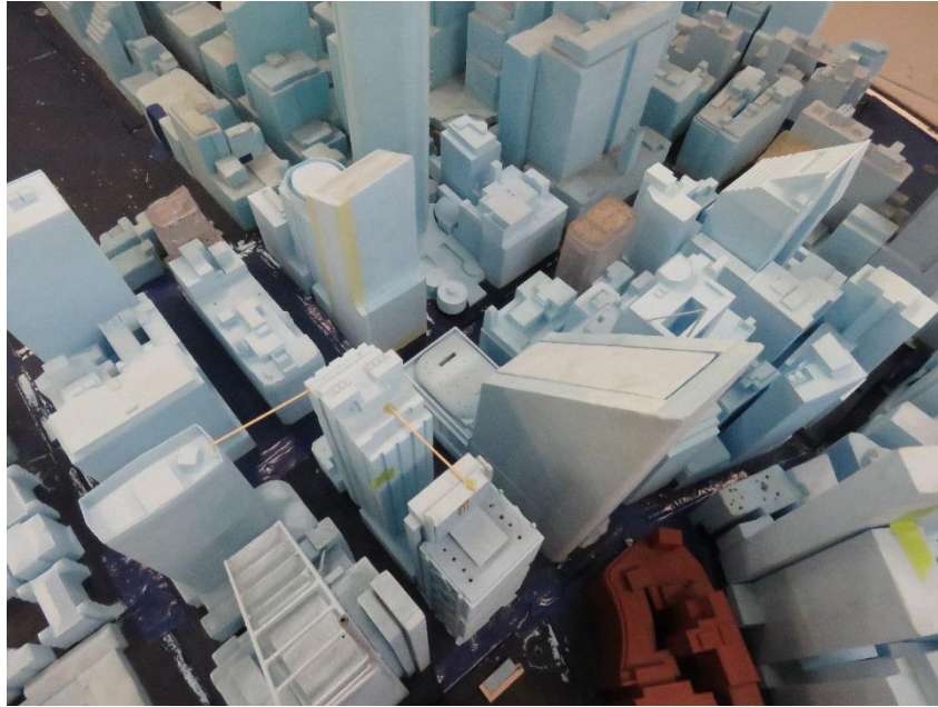
Figure 11: Close-up photograph of the wind tunnel model for Configuration B viewed from the north-east
