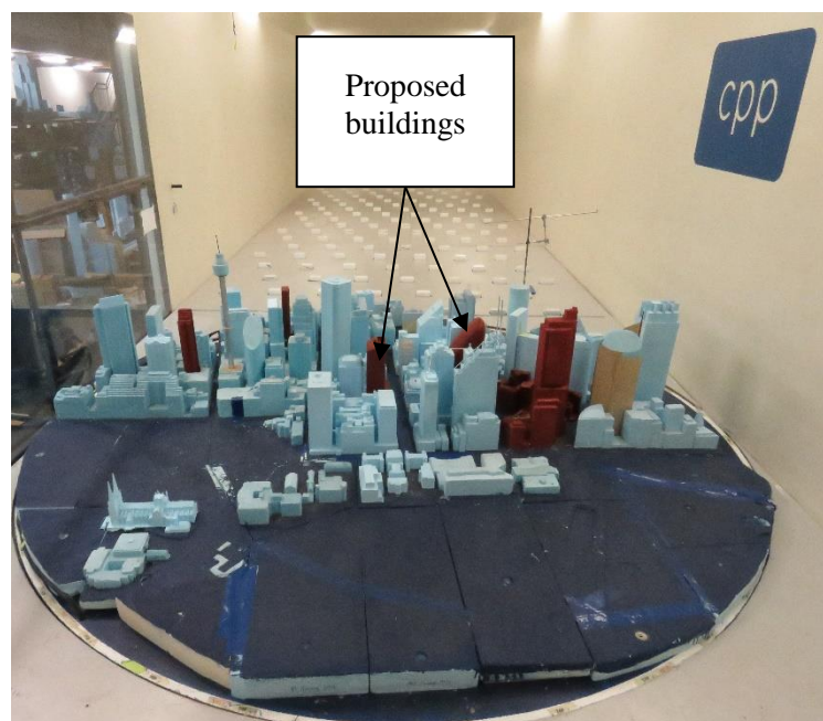
Figure 10: Photograph of the proposed configuration model in the CPP wind tunnel viewed from the east
