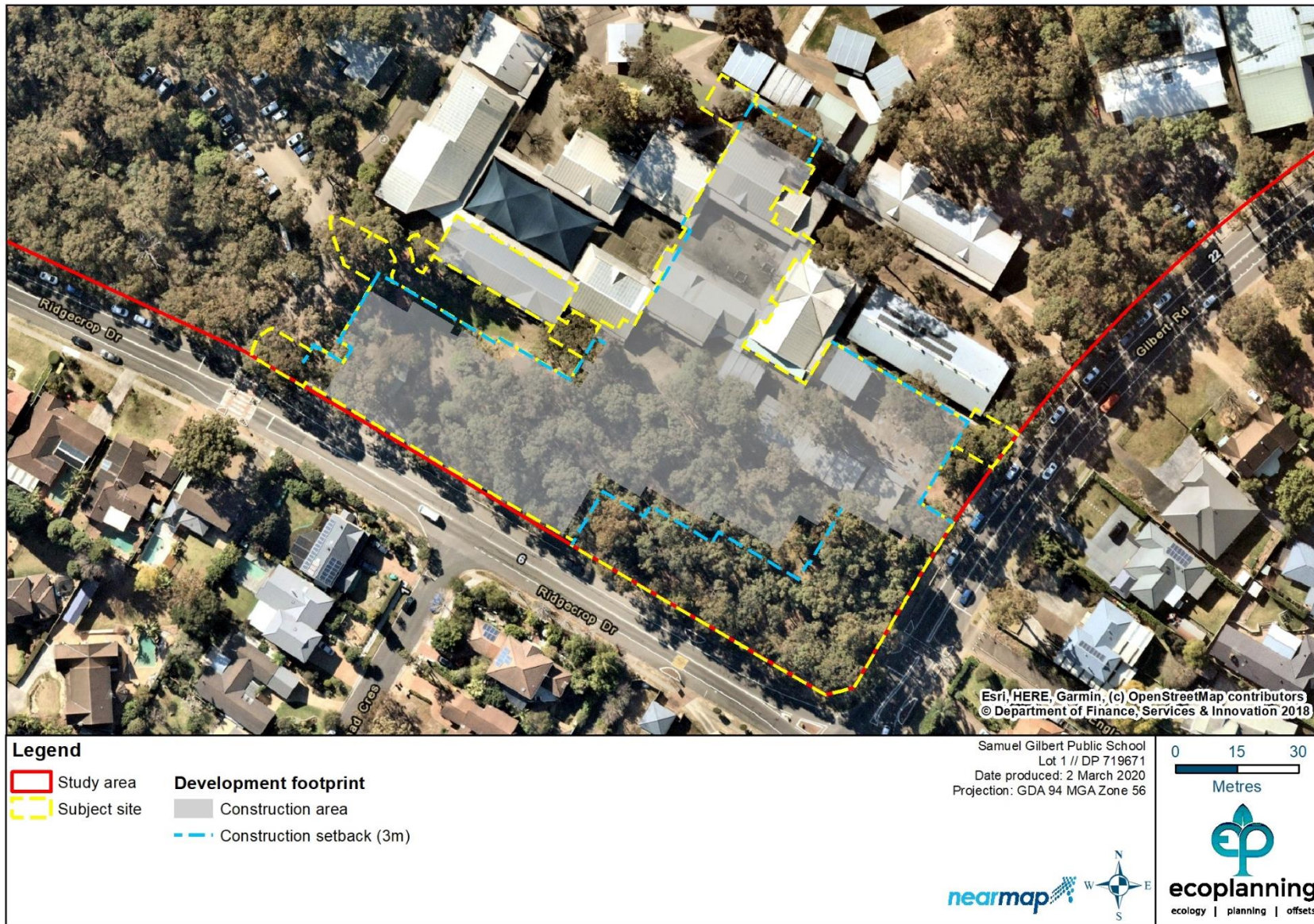
Figure 1.3: Development footprint, including construction setback.
