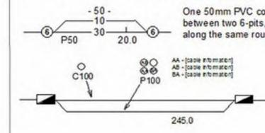
One 50mm PVC conduit (P50) containing a 50-pair and a 10-pair cable between two 6-pits, 20.0m apart, with a direct buried 30-pair cable along the same route.
