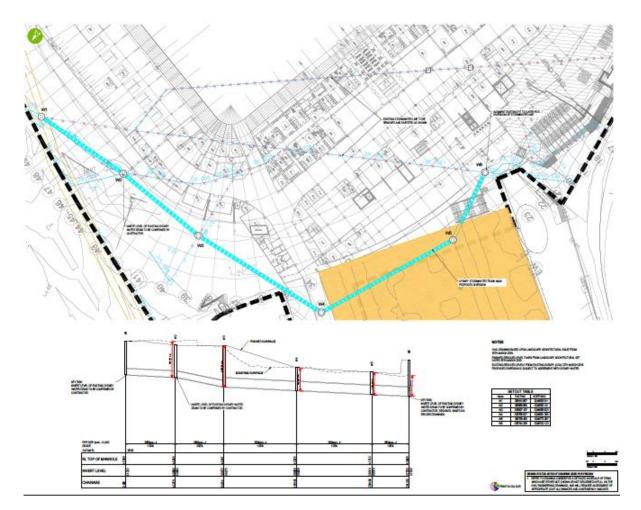
Figure 2: Stormwater Concept Location and long section
