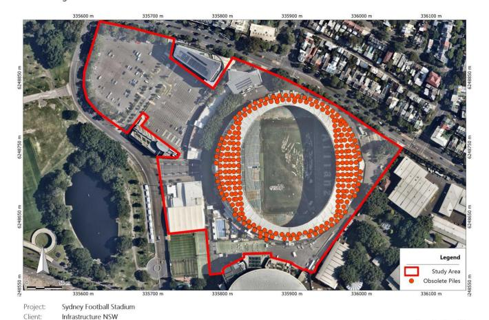
Figure 1 Demolition of below ground structures
