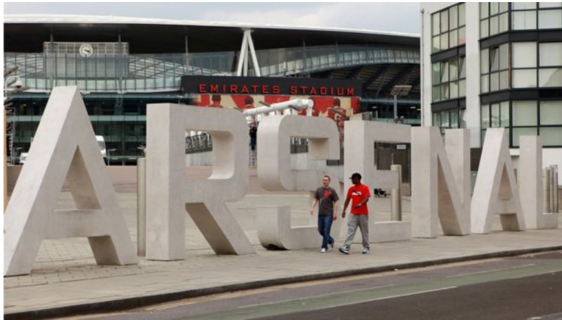
Example of use of aesthetic signage as vehicle intrusion barrier
