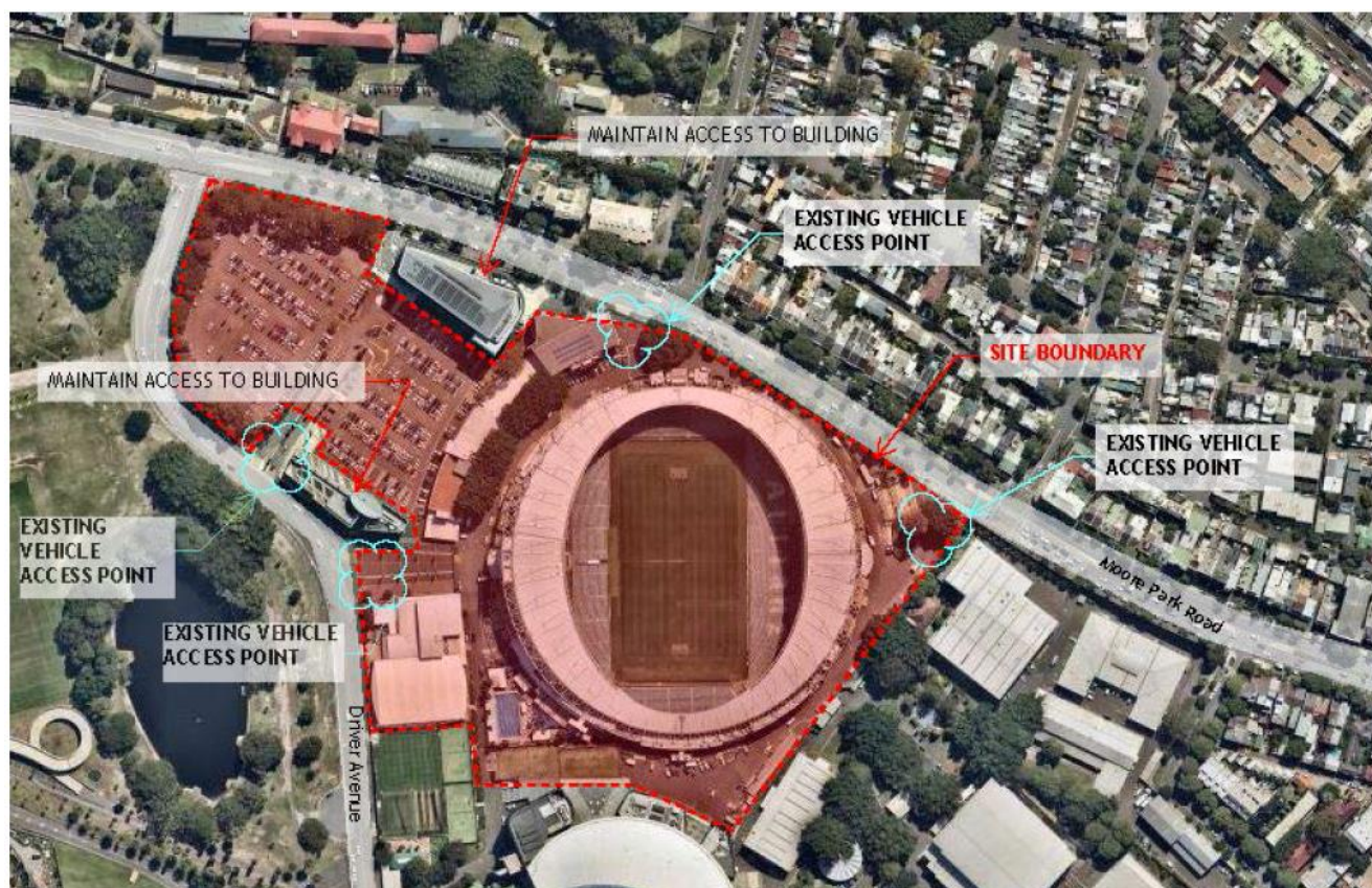
Figure 40 Vehicle access points for demolition phase
