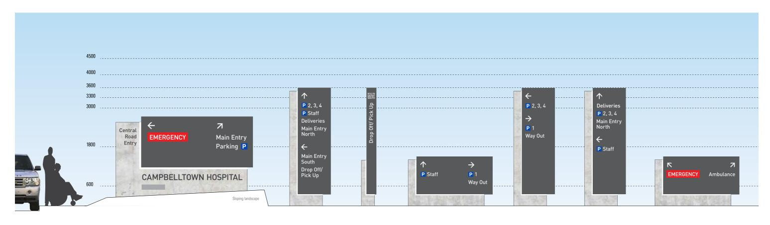
SITE ENTRY MARKER AND DIRECTIONAL 4200mm W x 2300mm (min) H + slope of landscape cap height directions: 140mm cap height campbelltown hospital: 180mm cap height entry name: 115mm PRIMARY VEHICULAR DIRECTIONAL 3600mm H x 1250mm W cap height: 115mm DESTINATION MARKER
