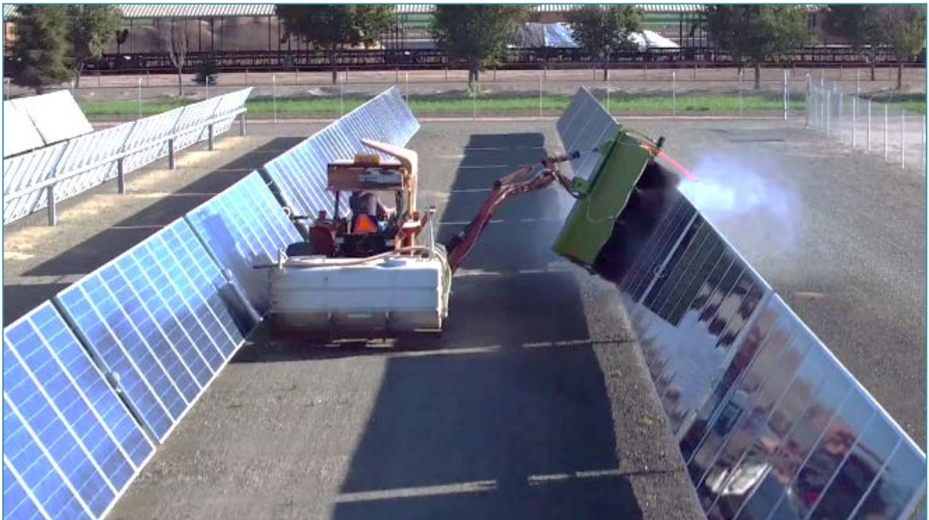
Figure 4 Sample Module Cleaning Procedures
