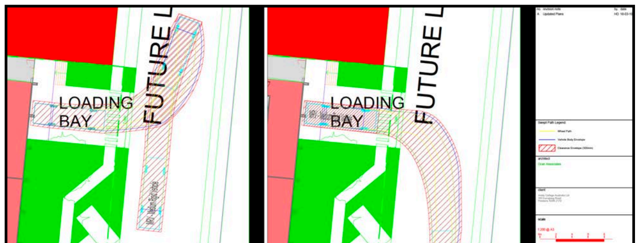
FIGURE 7.3 (above): Swept path analysis loading bay serving secondary school (Source: Appendix E of Traffic report )
