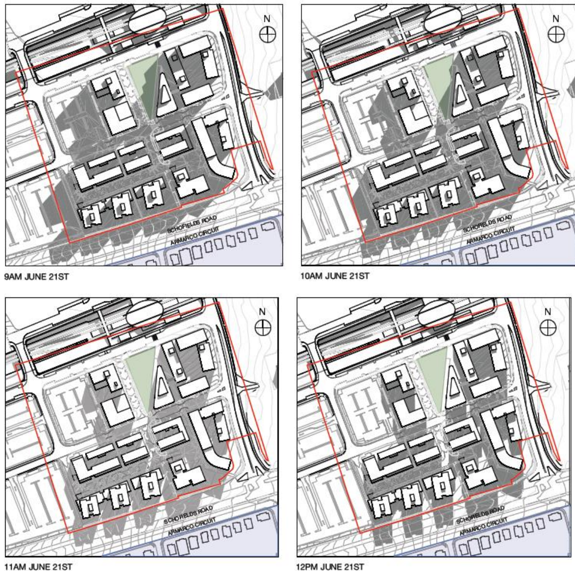
Figure 7: Solar analysis showing overshadowing from buildings mid winter 9am to 2pm.
