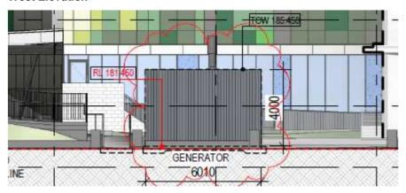
Figure 2 **Elevation view of the Generator enclosure**
