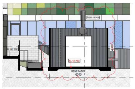
Figure 3 Section view of the Generator enclosure (with generator in centre)
