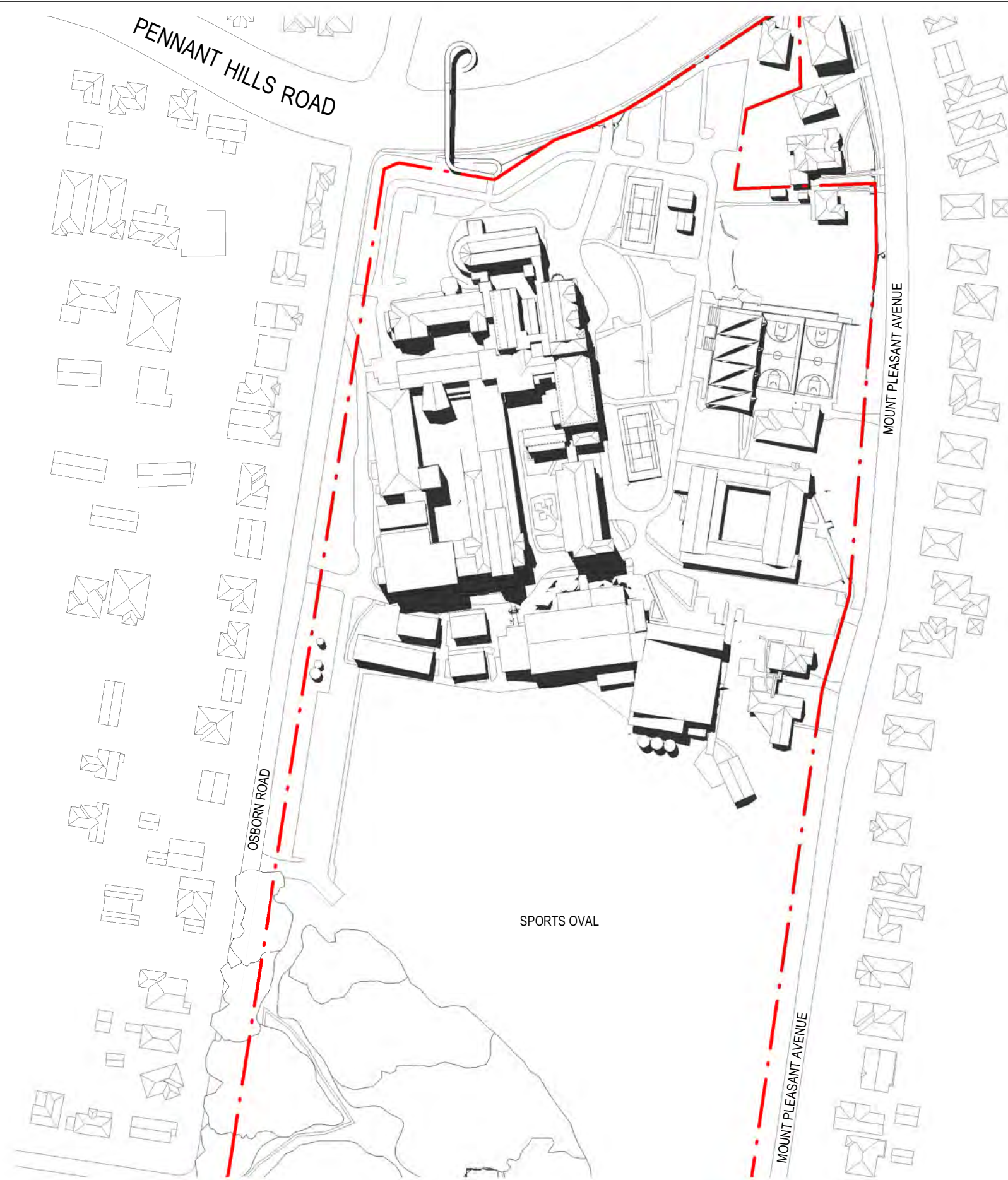
4 EXISTING SHADOW DIAGRAMS - 1pm EQUINOX 1:2000
