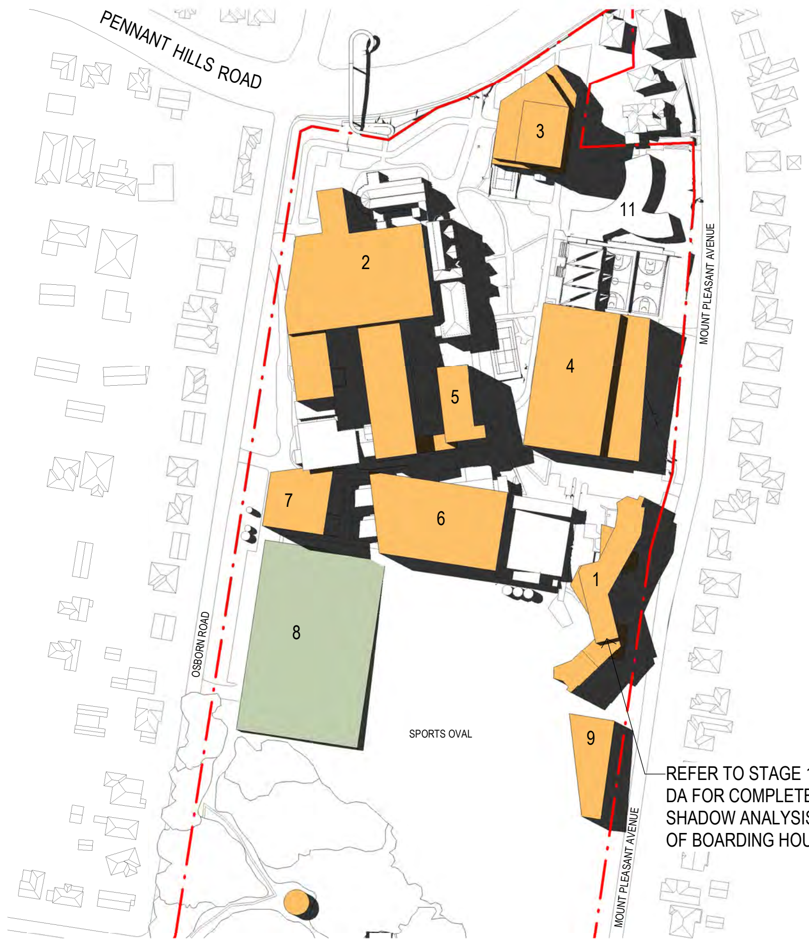
1 PROPOSED SHADOW DIAGRAMS - 3pm EQUINOX 1:2000
