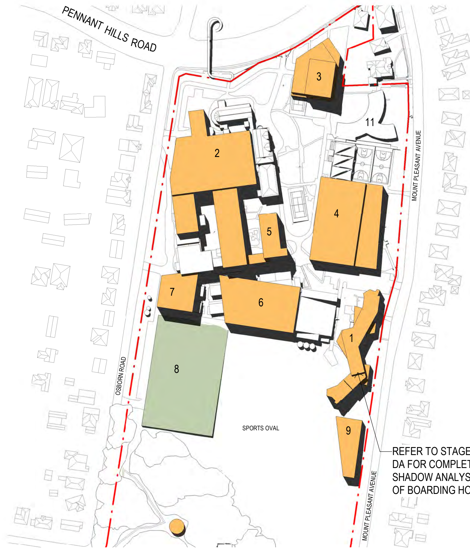
3 PROPOSED SHADOW DIAGRAMS - 1pm EQUINOX 1:2000
