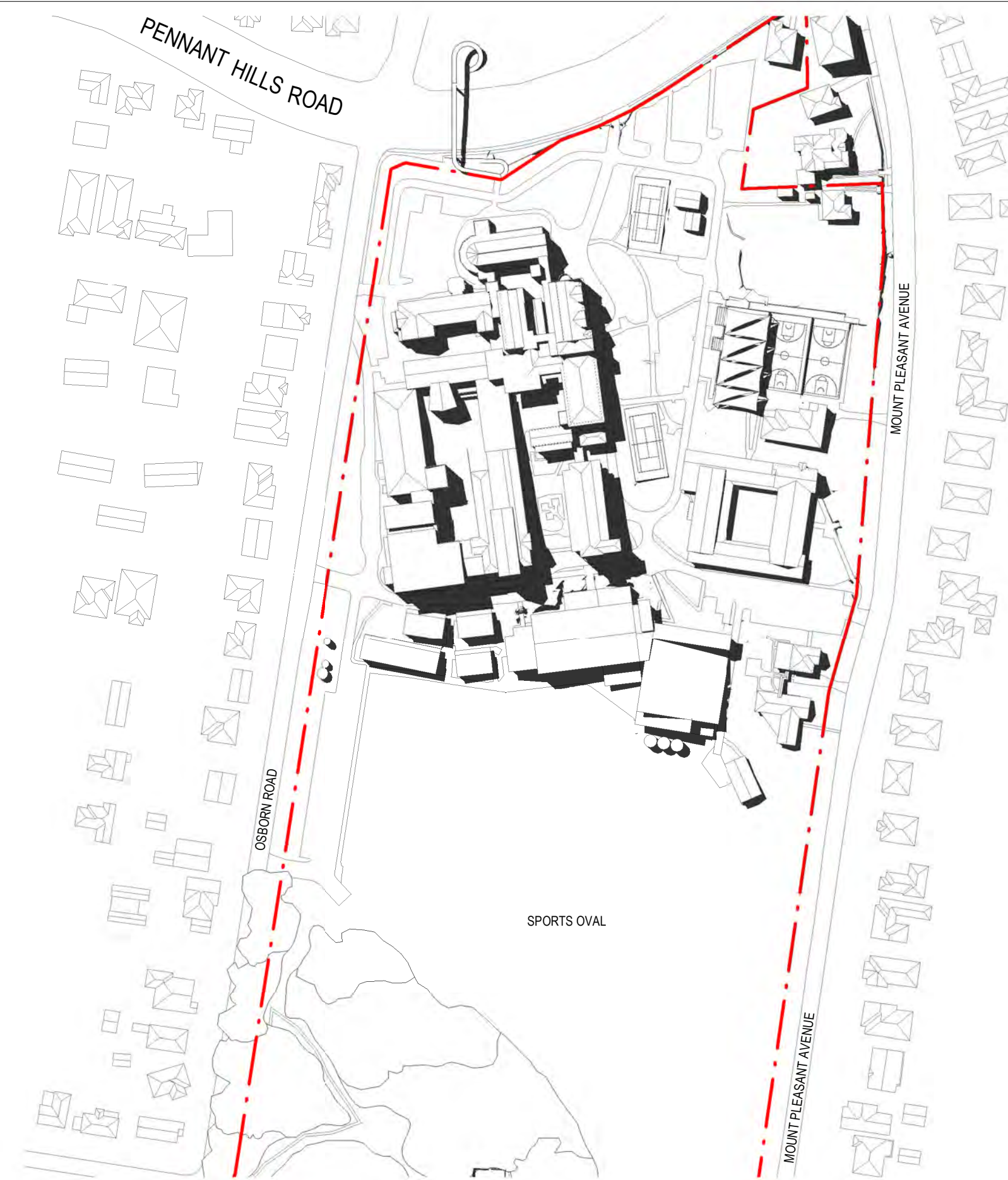
2 EXISTING SHADOW DIAGRAMS - 2pm EQUINOX 1:2000
