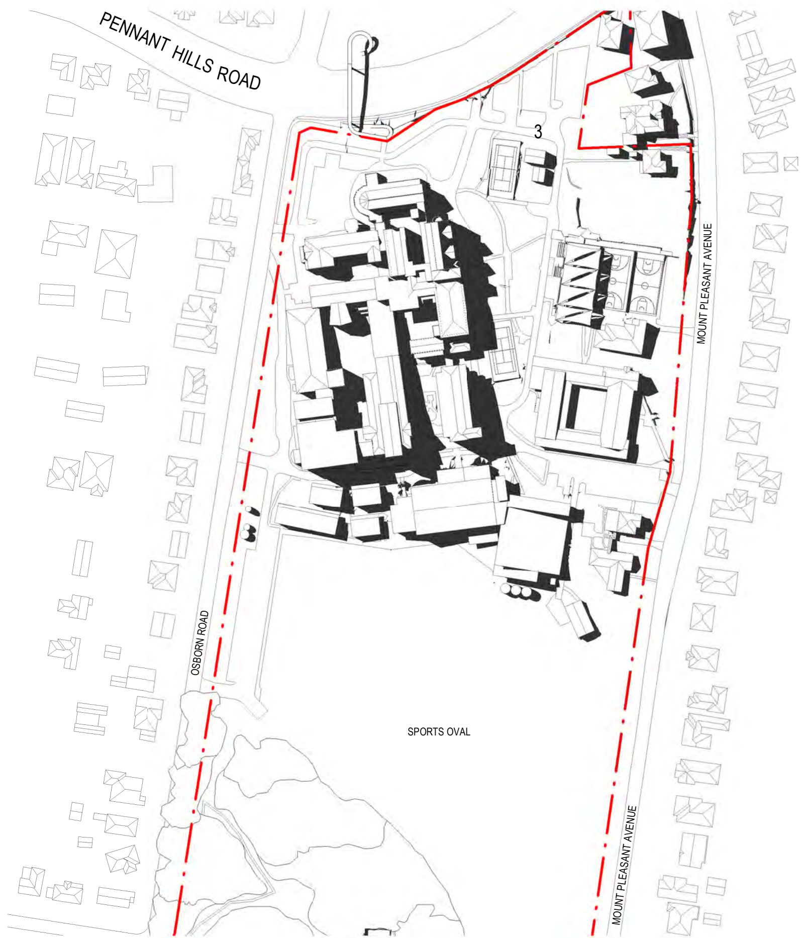
2 EXISTING SHADOW DIAGRAMS - 3pm EQUINOX 1:2000
