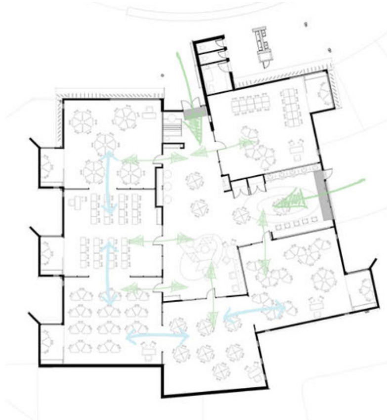
Figure 29: Typical Primary School Block Access & Operability Diagram
