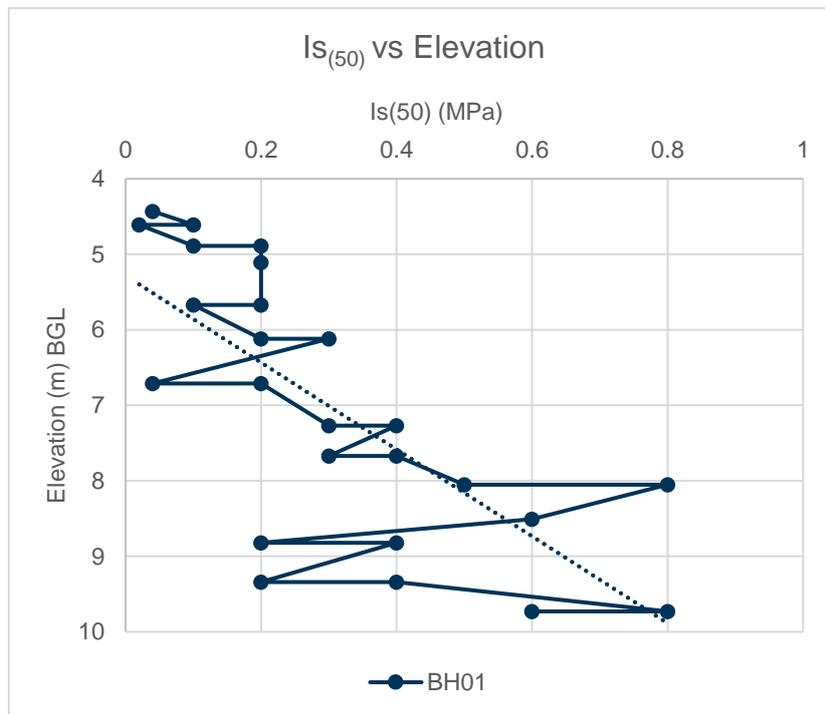
**Figure 10-1 Comparison of  $I_{s(50)}$  Values vs Elevation Depth for BH01**
