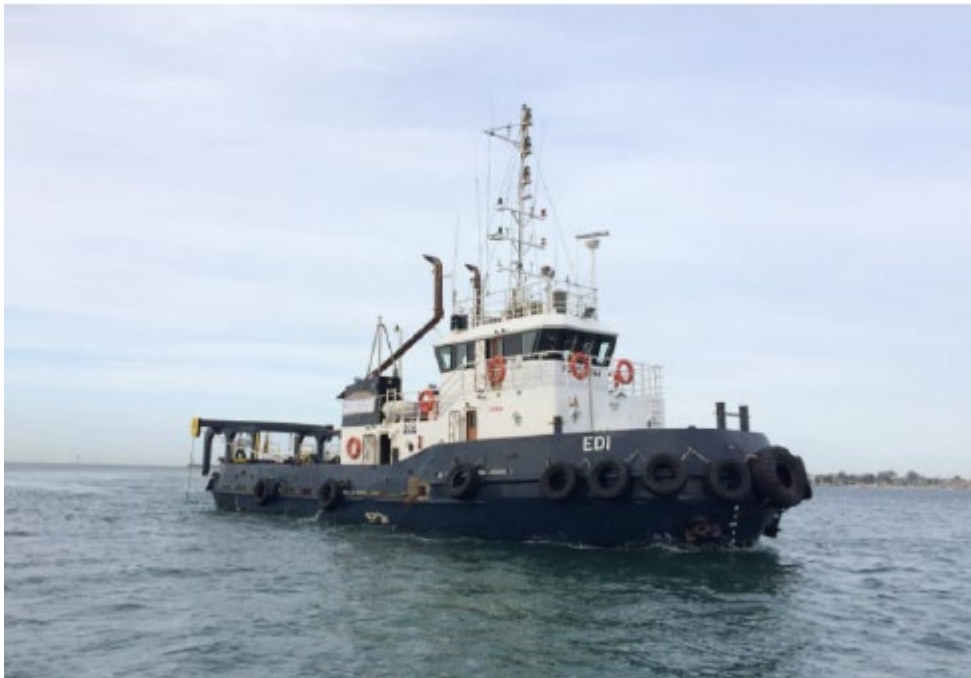
Figure 5. Vessel with sweep bar example.
