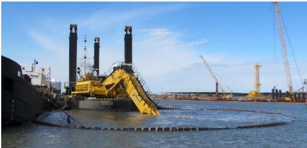
Figure 2. Typical moonpool arrangement
