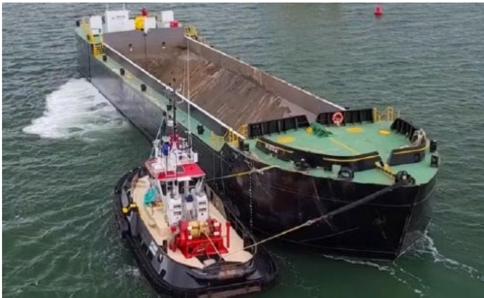
Figure 4. Hip Tow zone arrangement
