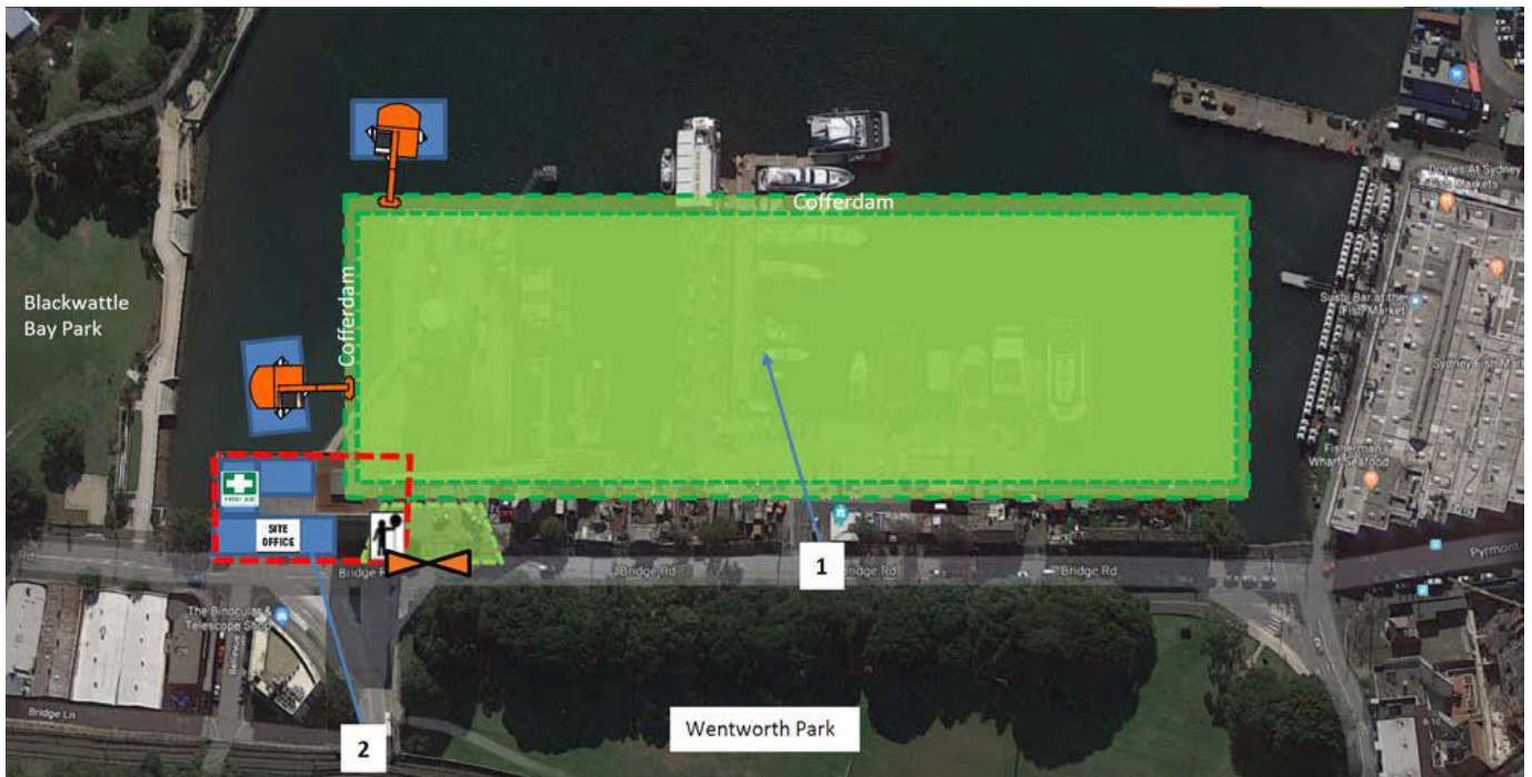
Figure 5: Site Activities for Stage 2 (Main Works) – substructure works and cofferdam – staging program
