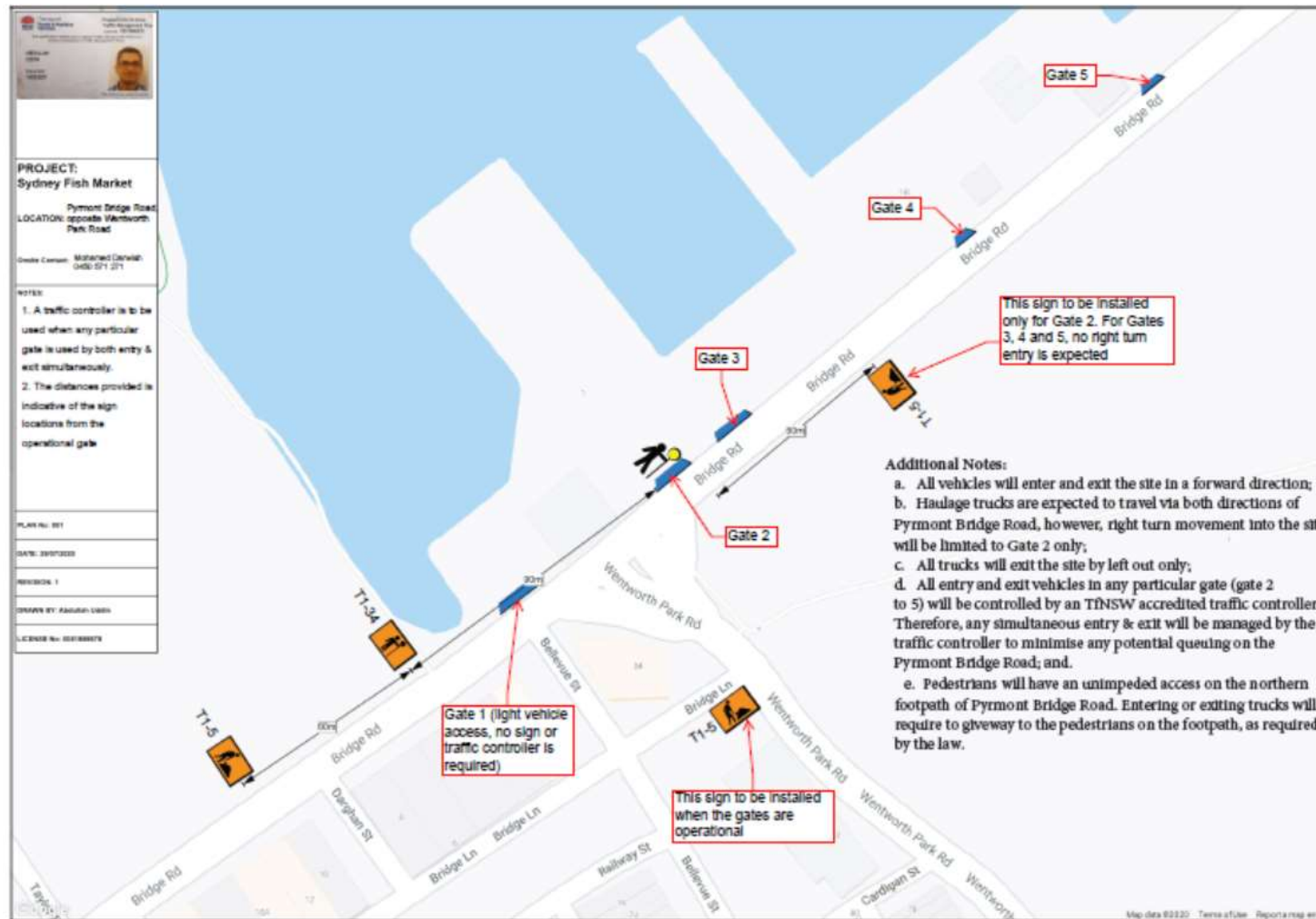
Figure 6 - Traffic Control Plans for general operating site conditions at 1a, b & c Bridge Road
