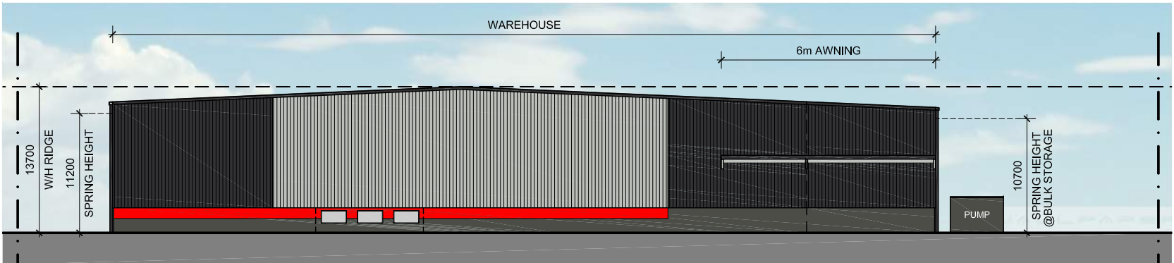
4 NORTH ELEVATION 200 Scale 1:500
