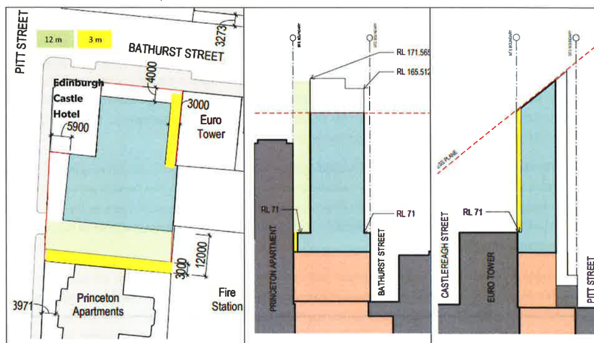
Figure 26 | The setbacks for the development showing plan view (left) and section views (middle and right) (source: RtS).
