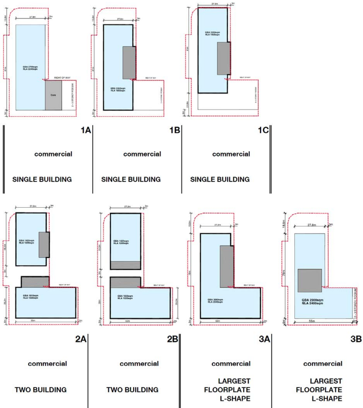
Figure 36: Excerpt from Section 5.1 of the Victoria Cross Urban Design Report showing the floor plate studies of the different design options explored for the Victoria Cross OSD site.
