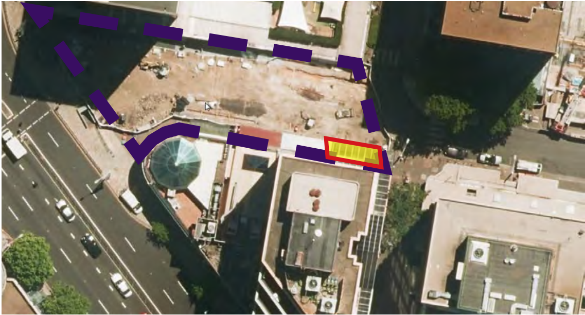
Overlay of extent of shadow created by the OSD concept SSDA building envelope on Brett Whiteley Plaza at 12pm June 21st
