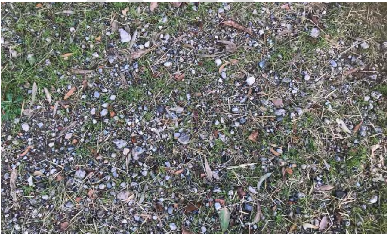
Photograph 18: gravel containing crushed demolition waste observed surrounding the gymnasium along the western site boundary
