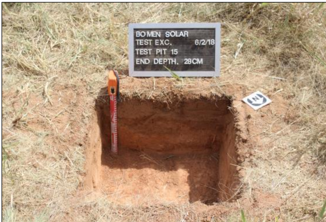
Plate 26 Representative soil profile in Phase 1 test pit TP#15 (Source: AECOM 2018)
