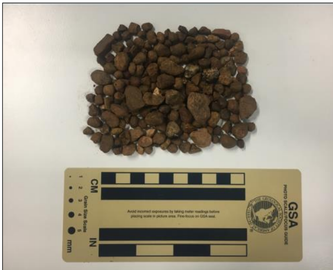
Plate 27 Ironstone and quartz gravel from TP#3 (Source: AECOM 2018)
