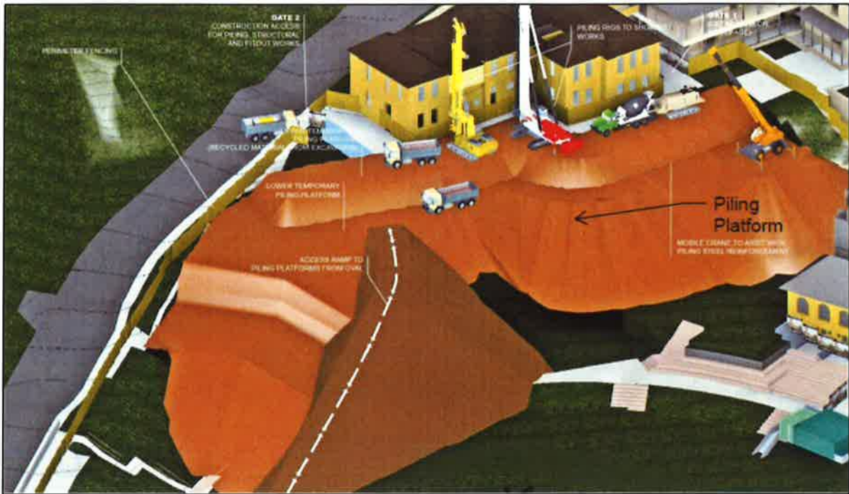
Figure 13 | Proposed piling platform during excavation (Source: Applicant's RtS 2019).
