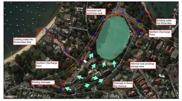
Figure 5 Pre-development stormwater conditions
