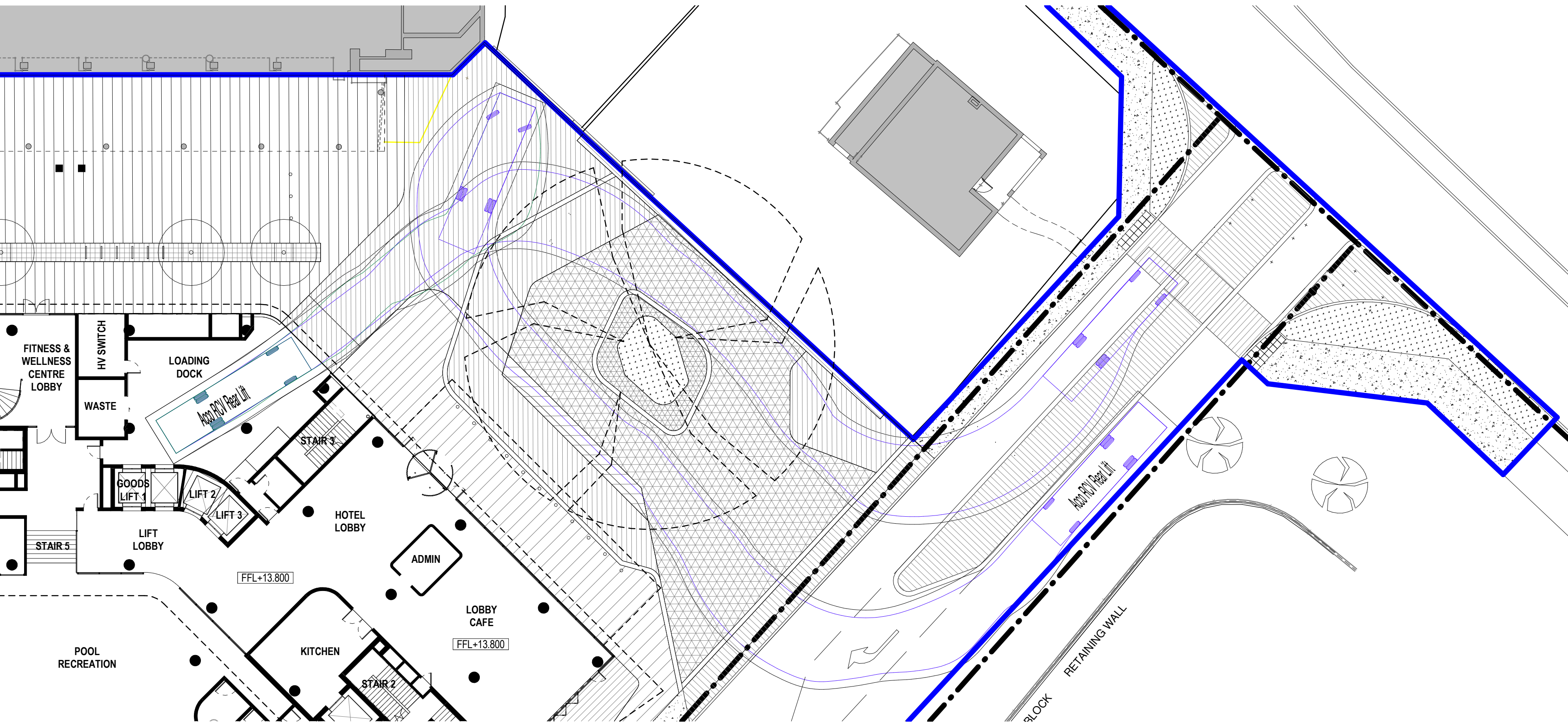
2 WASTE - VEHICLE ENTERING & EXITING 1:200
