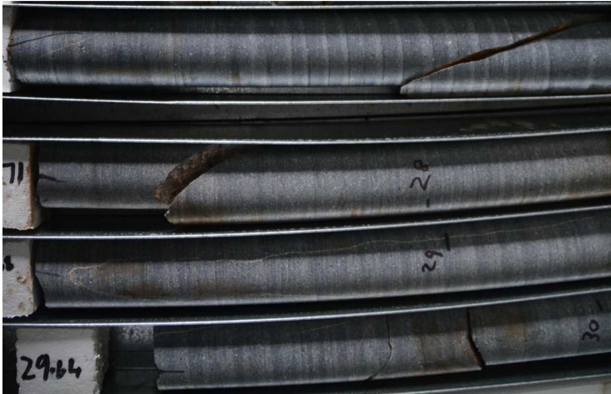
Plate 2.1 Drill Core displaying the dark natural colour of the rhyodacite within the Site (Ref: E958A_016)
