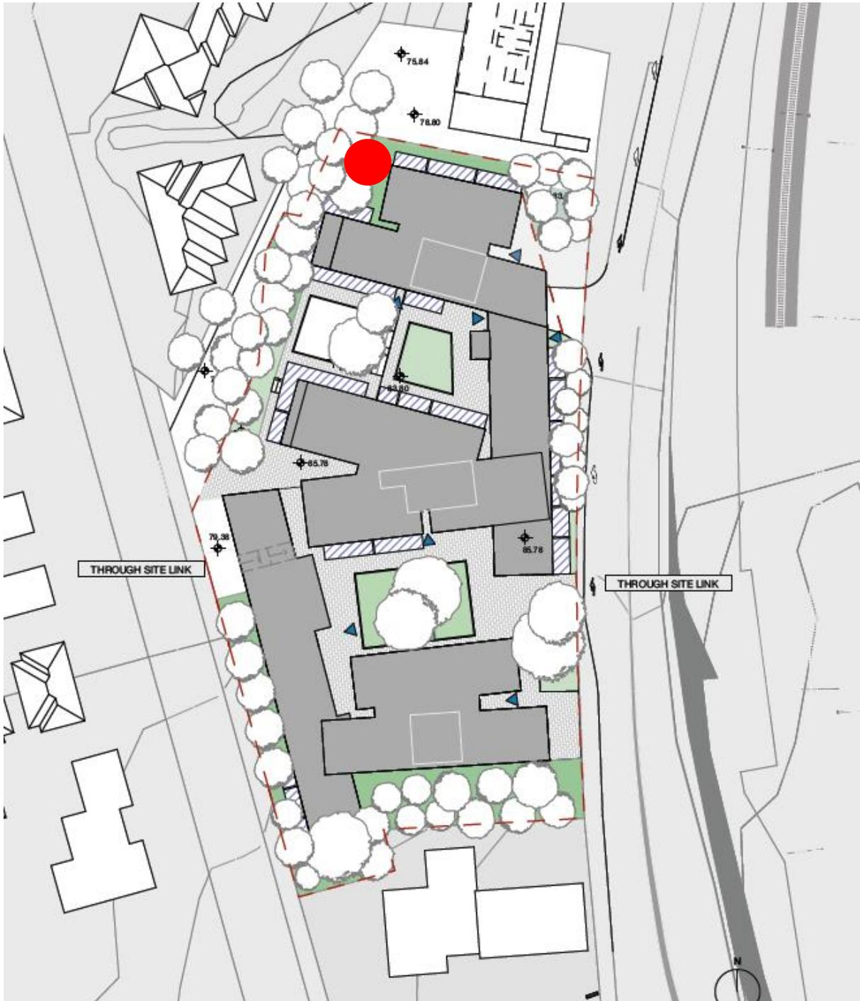
Figure 9: Possible Location of stormwater bioretention system in red in the north-western corner of the site.
