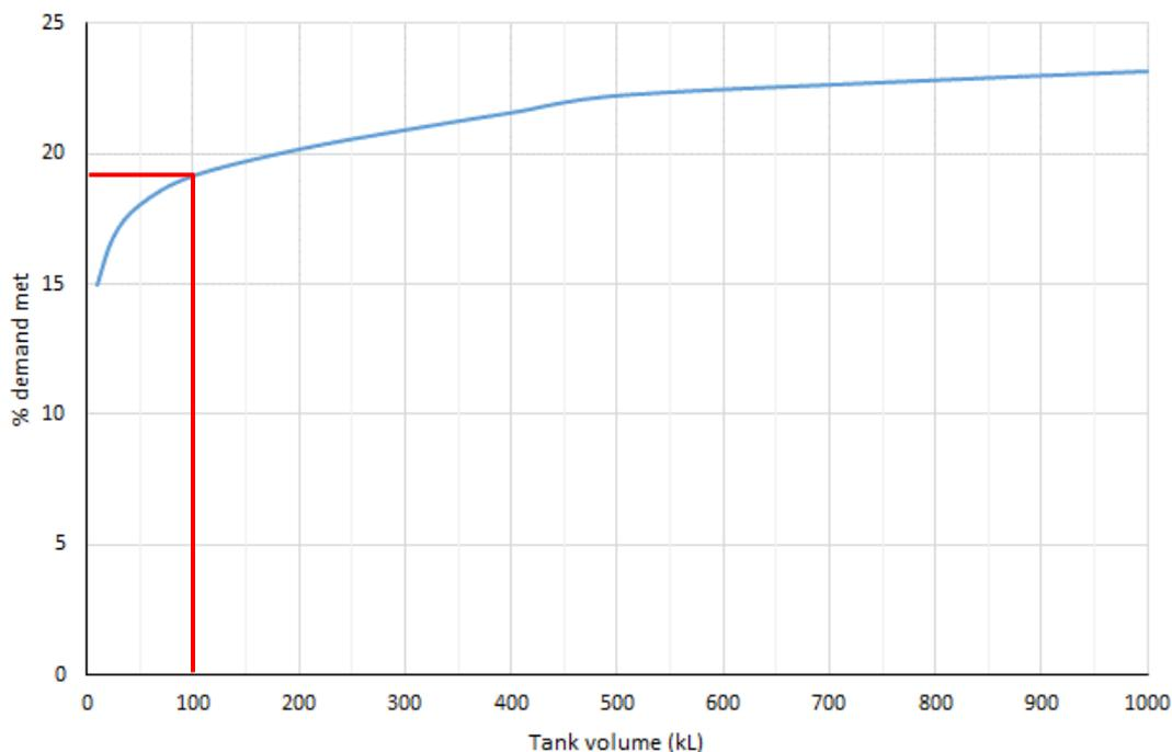
**Figure 7. Rainwater tank sizing curve**
