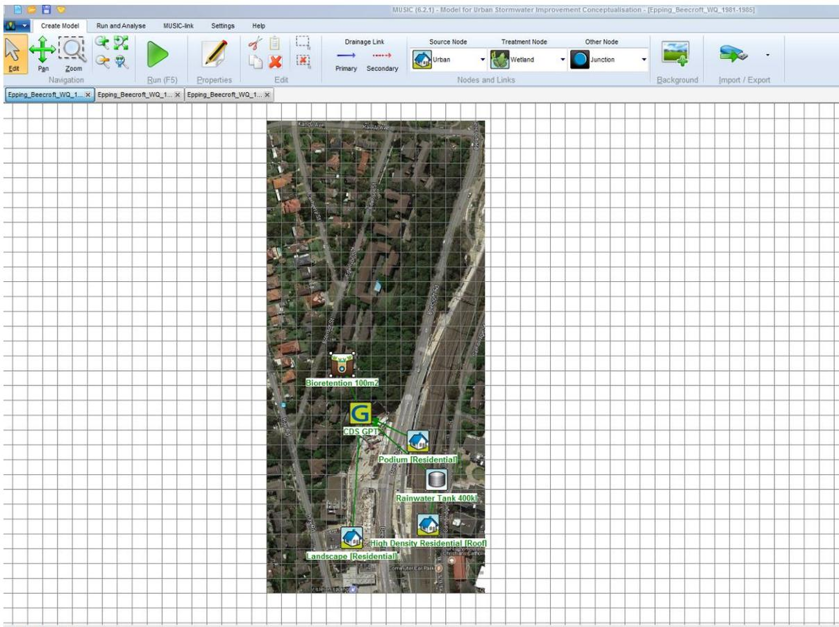
**Figure 8: MUSIC model schematic of proposed site development at Epping**
