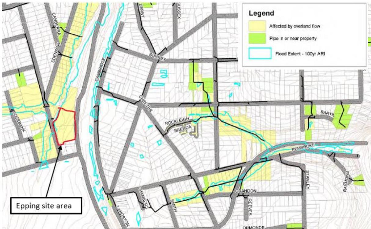
Figure 5: Map of properties affected by Overland Flow (100 year ARI) as detailed in the Hornsby Overland Flow Study (Cardno 2010).
