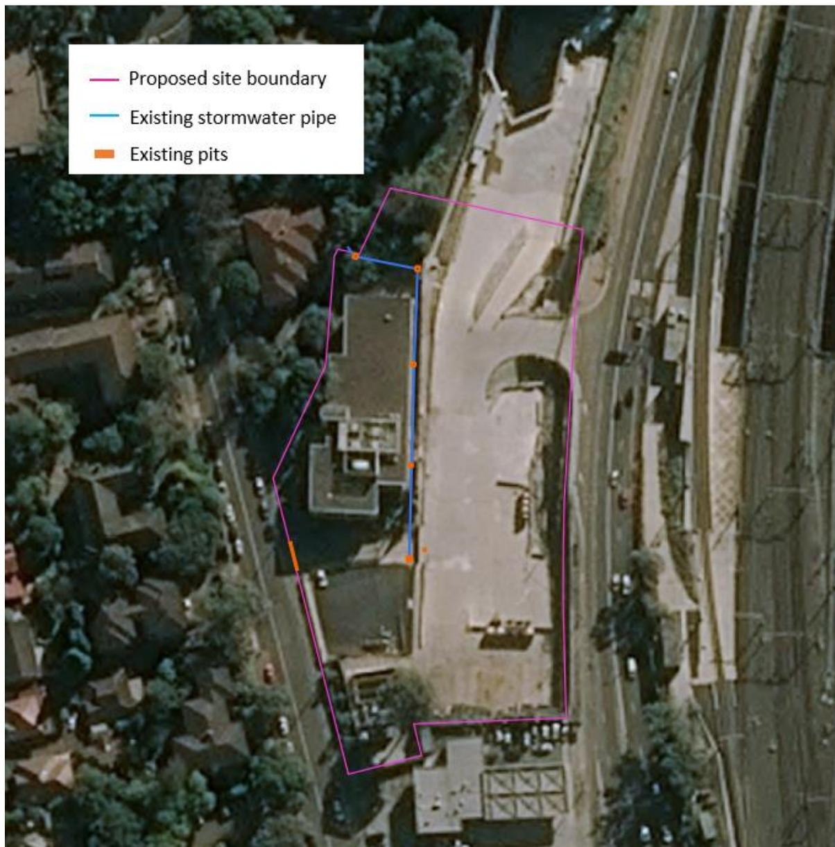
Figure 2: Proposed development with existing drainage (aerial image from Bing)
