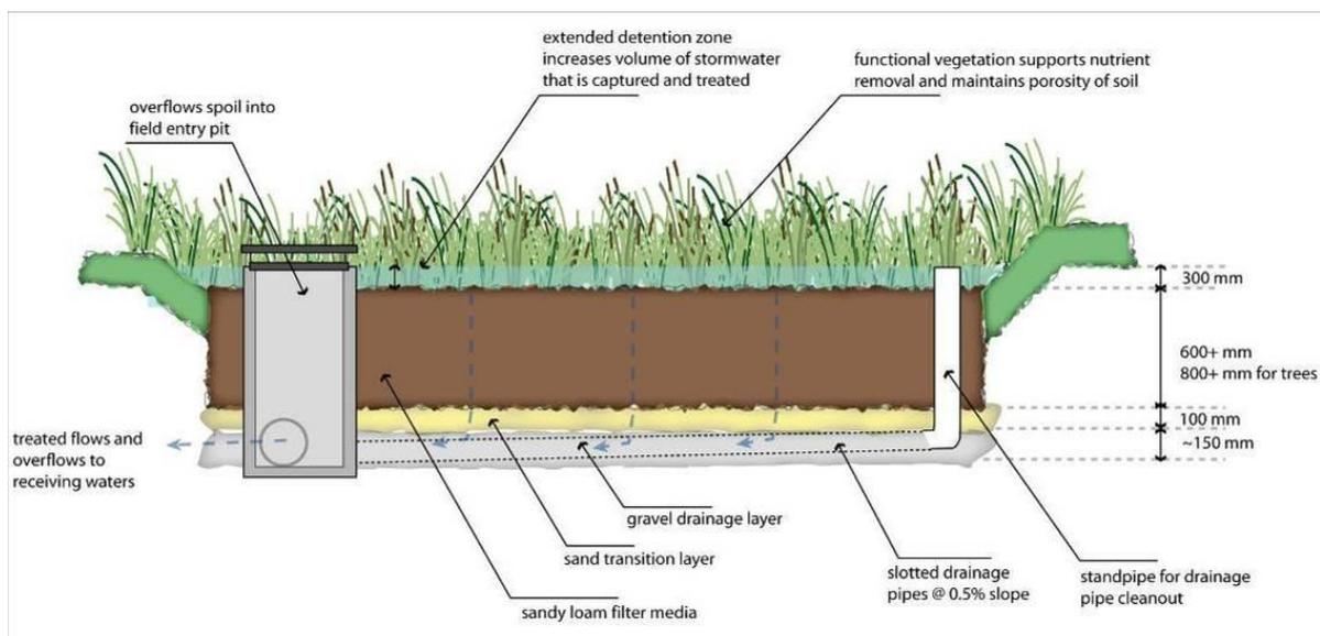
**Figure 10: Schematic section through a typical bioretention system**
