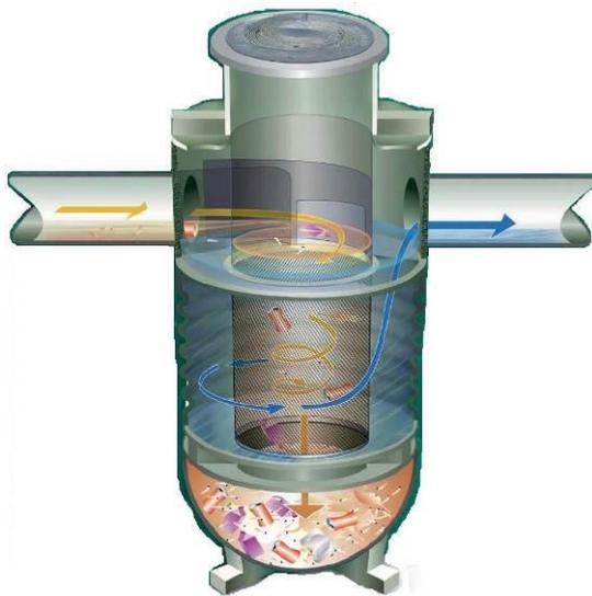
Figure 12: Illustrative section through a Rocla CDS 'Nipper'
