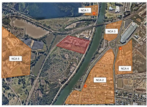
Figure 1 Project area (□), monitoring positions (★), and noise catchment areas (□)
