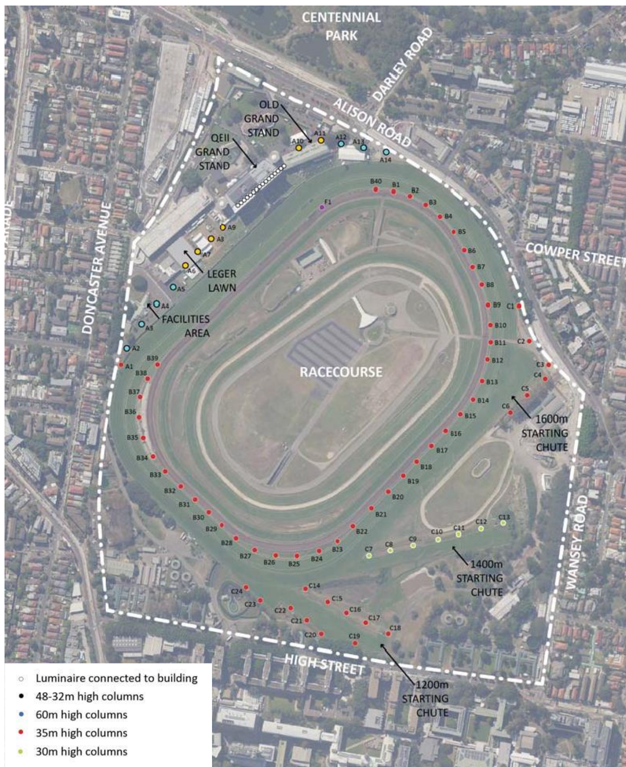
Figure 17 Trackside lighting design – Heights of light columns
