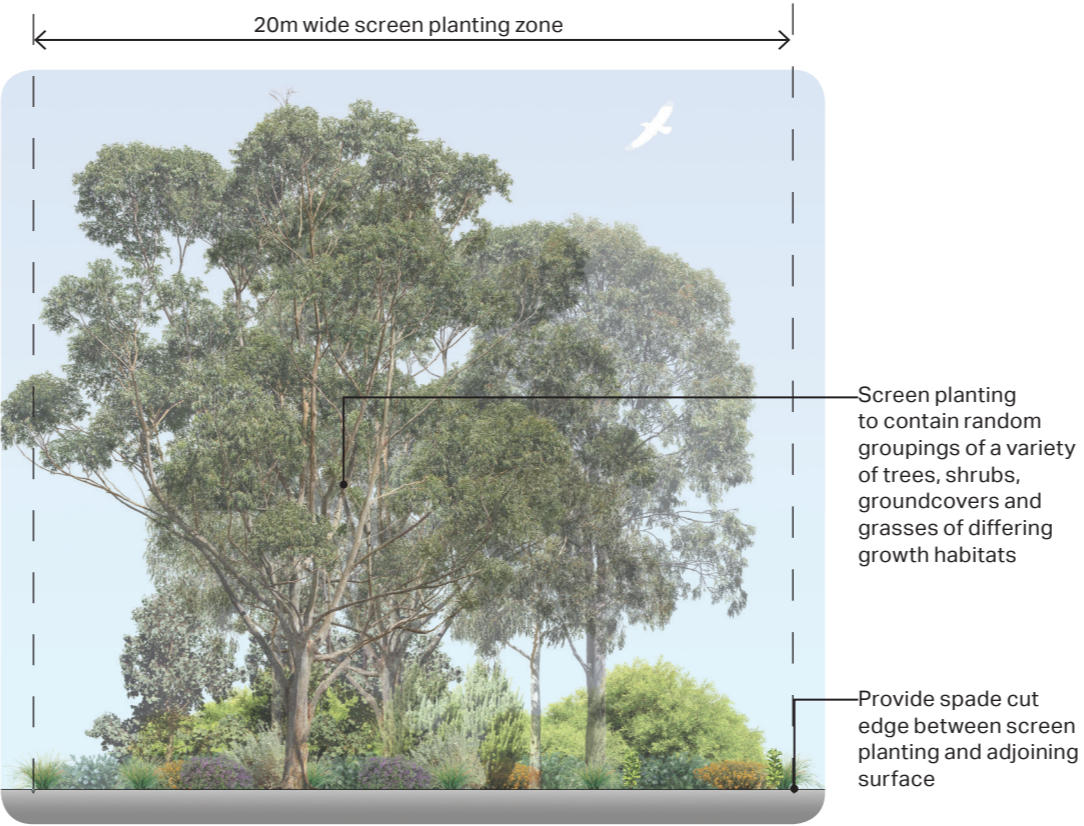
DETAIL 2: SCREEN PLANTING - TYPICAL SECTION 1:200
