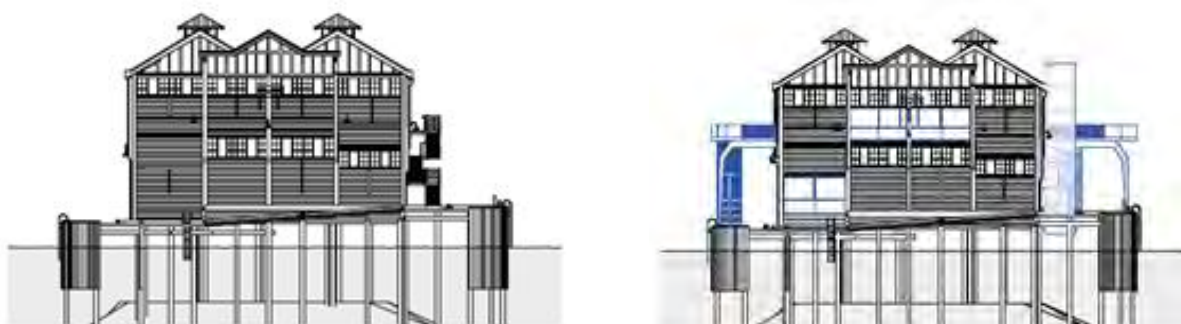
Figure 8 - Existing and proposed north elevation to Pier 2/3 (proposed alterations shown in blue)
