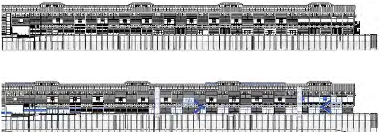
Figure 6 - Existing and proposed east elevation to Wharf 4/5 (proposed alterations shown in blue)
