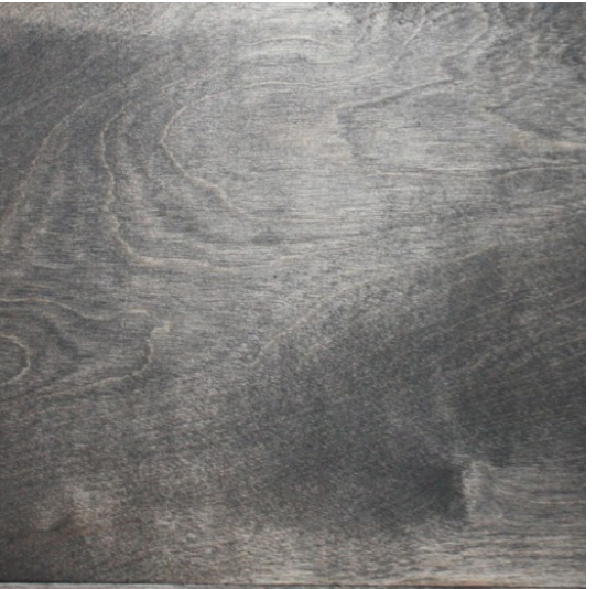
Figure 50: TC01 Timber Cladding Type 1 Birch Plywood, sheets cut down to 6 pieces of varying sizes to create wall pattern, 3 shades of black and 3 levels of sheen.
