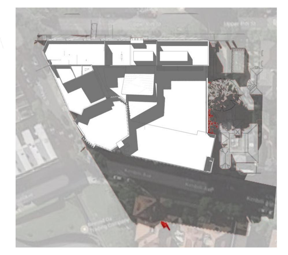
Shadow Diagram 1pm June 21st Scale: 1:500
