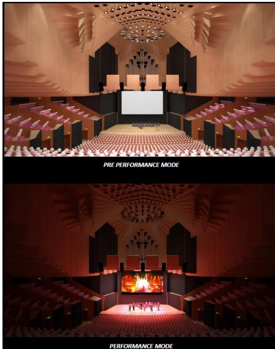
Figure 72: Concert Hall Concept Design – Acoustic Banners and Drapes (from circle)
