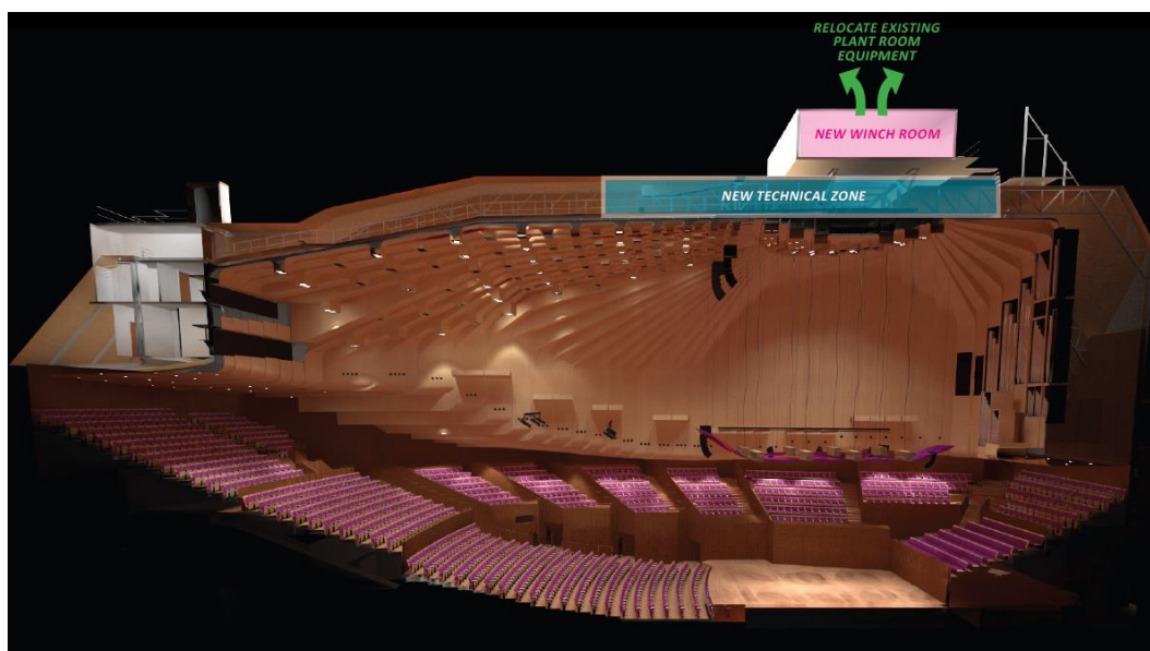
Figure 90: Concert Hall Design Development – Section Showing Changes Proposed to Technical Zone
