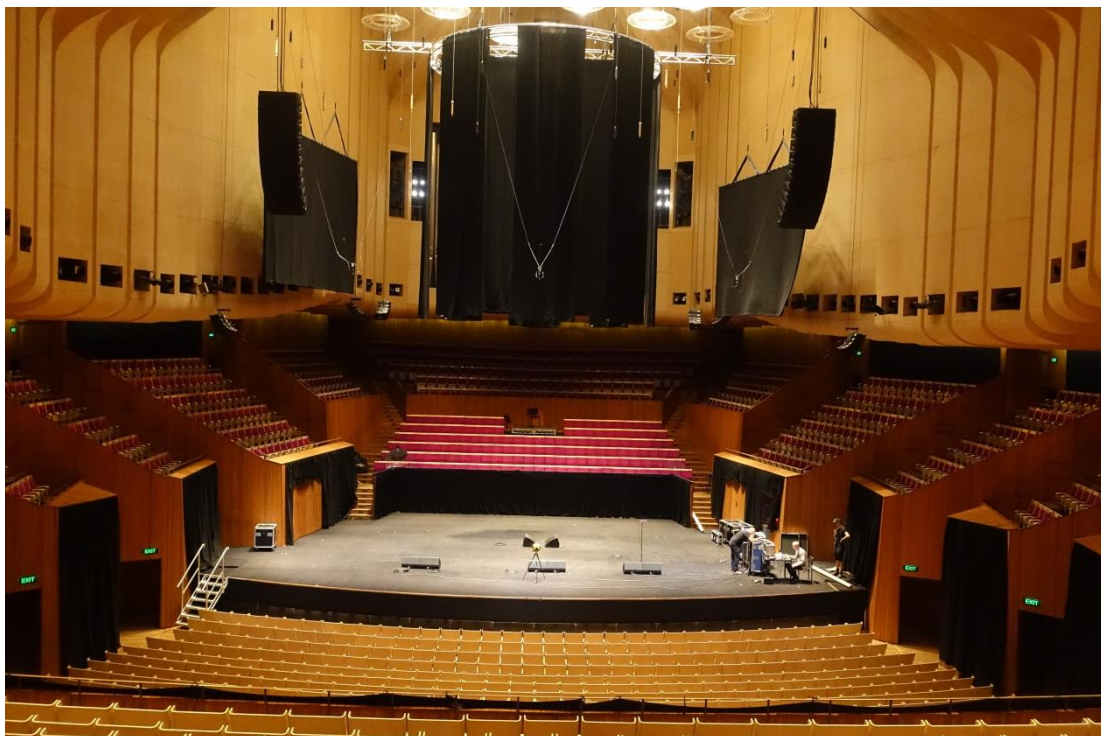
Figure 17: Concert Hall set up for acoustic testing of absorption drapes, Müller-BBM acousticians and test equipment on stage
