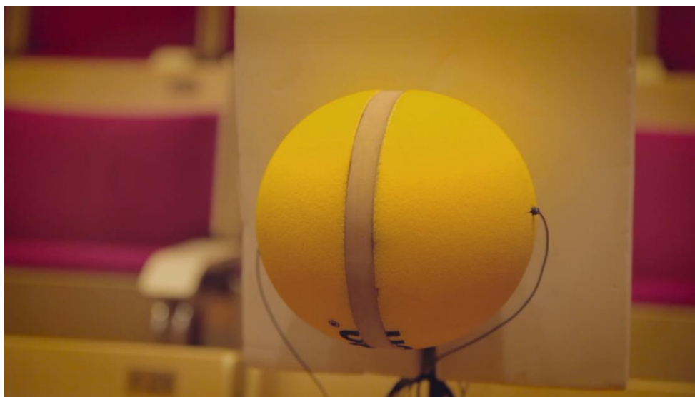
Figure 6: Acoustical Measurement Dummy in Concert Hall Seats
