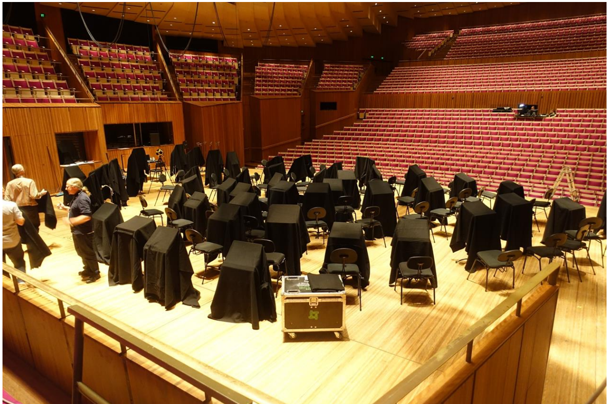
Figure 11: Stage set up for acoustic measurements (sound source towards the left hand side, covers over music stands to simulate 'absorption' effect of orchestra)
