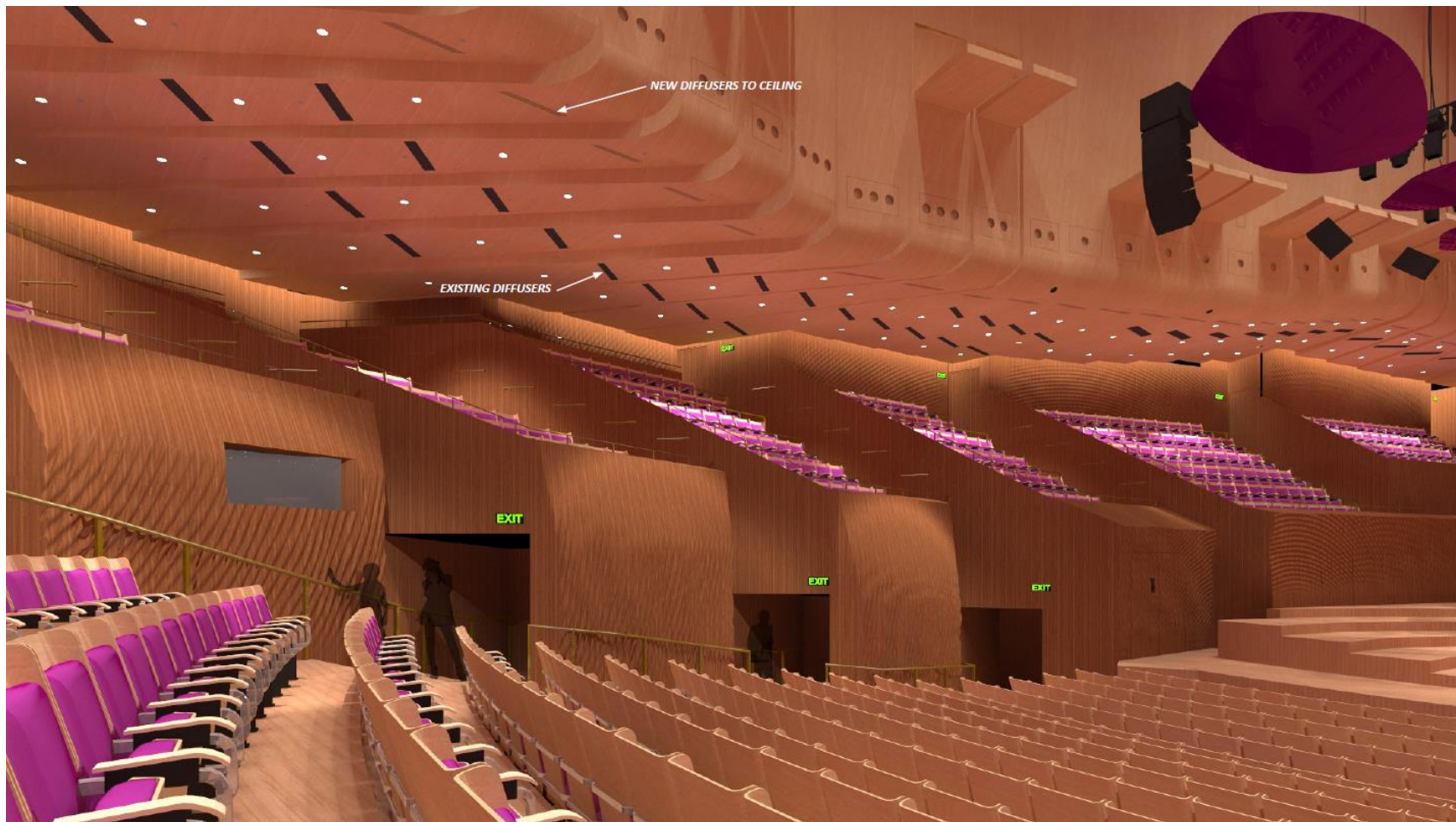
Figure 18: Render of proposed air conditioning diffuser slots locations/layout
