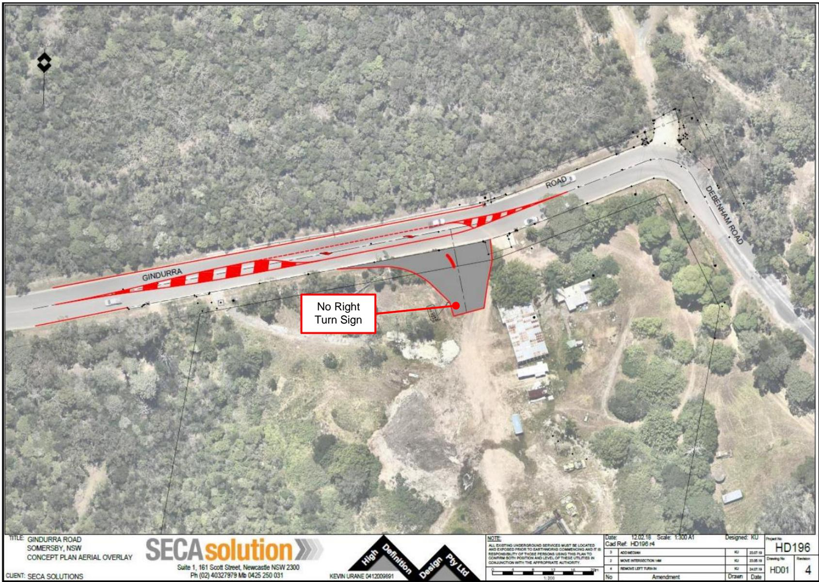
Figure 2: Upgrades of Gindurra Road and the Proposed Site Access Plan
