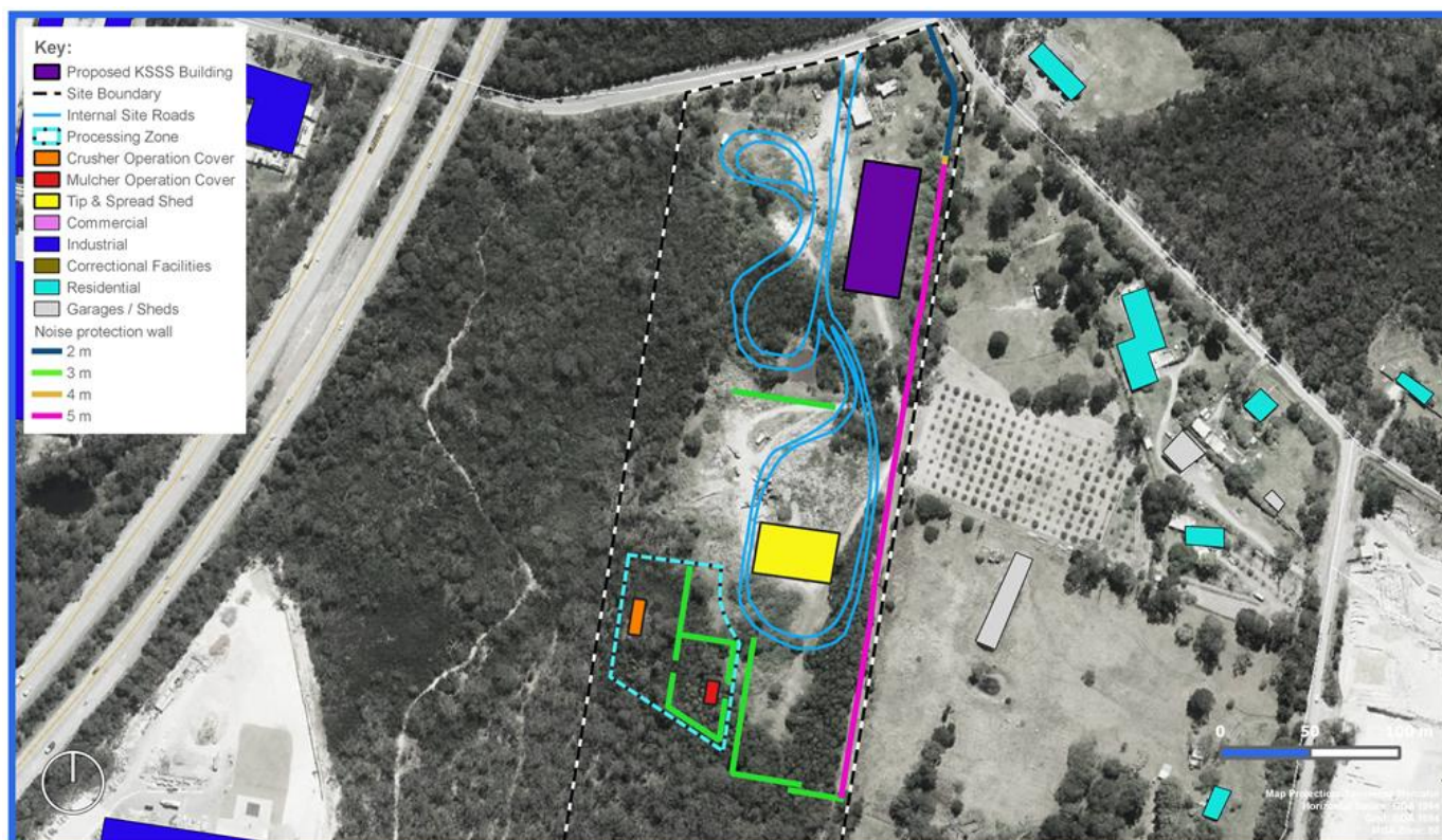
Figure 11.1. Recommended noise barrier locations, heights and extents to achieve compliance with the PNTLs.
